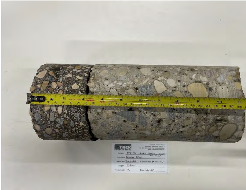
Photo 1: Pavement Core Sample at Test Hole TH23-21
