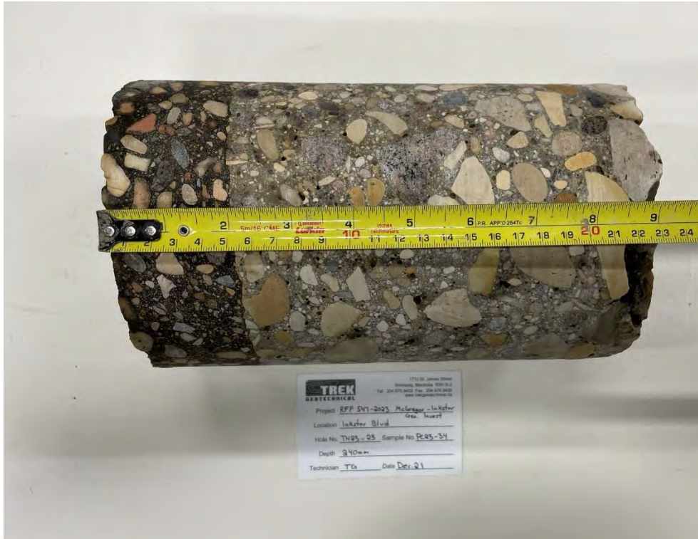
Photo 3: Pavement Core Sample at Test Hole TH23-23
