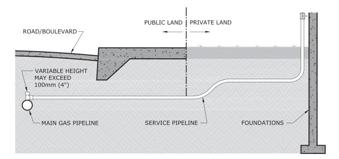
**IMPORTANT:** Gas pipelines are generally yellow in color; however, there are instances of other colors being used such as black, blue, orange, tan and green as an example. Caution when verifying must be observed and all pipes and cables excavated must be considered "operational" until verified by a Manitoba Hydro representative.
