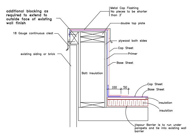
26 Gauge counter flashing complete with approx. 1/2" 45 degreee bottom kick out is to be installed over all membrane stripping. Terminate flashing about 1" above top of new roofing. Do not install any fasteners behind the cap flashing and use only lap joints. This is to allow easy removal for future repairs.
