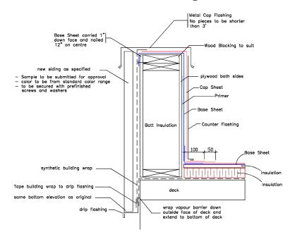
26 Gauge counter flashing complete with approx. 1/2" 45 degreee bottom kick out is to be installed over all membrane stripping. Terminate flashing about 1" above top of new roofing. Do not install any fasteners behind the cap flashing and use only lap joints. This is to allow easy removal for future repairs.
