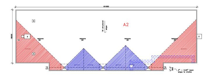
2% sloped type 2 EPS min 0.25" in direction of arrows
