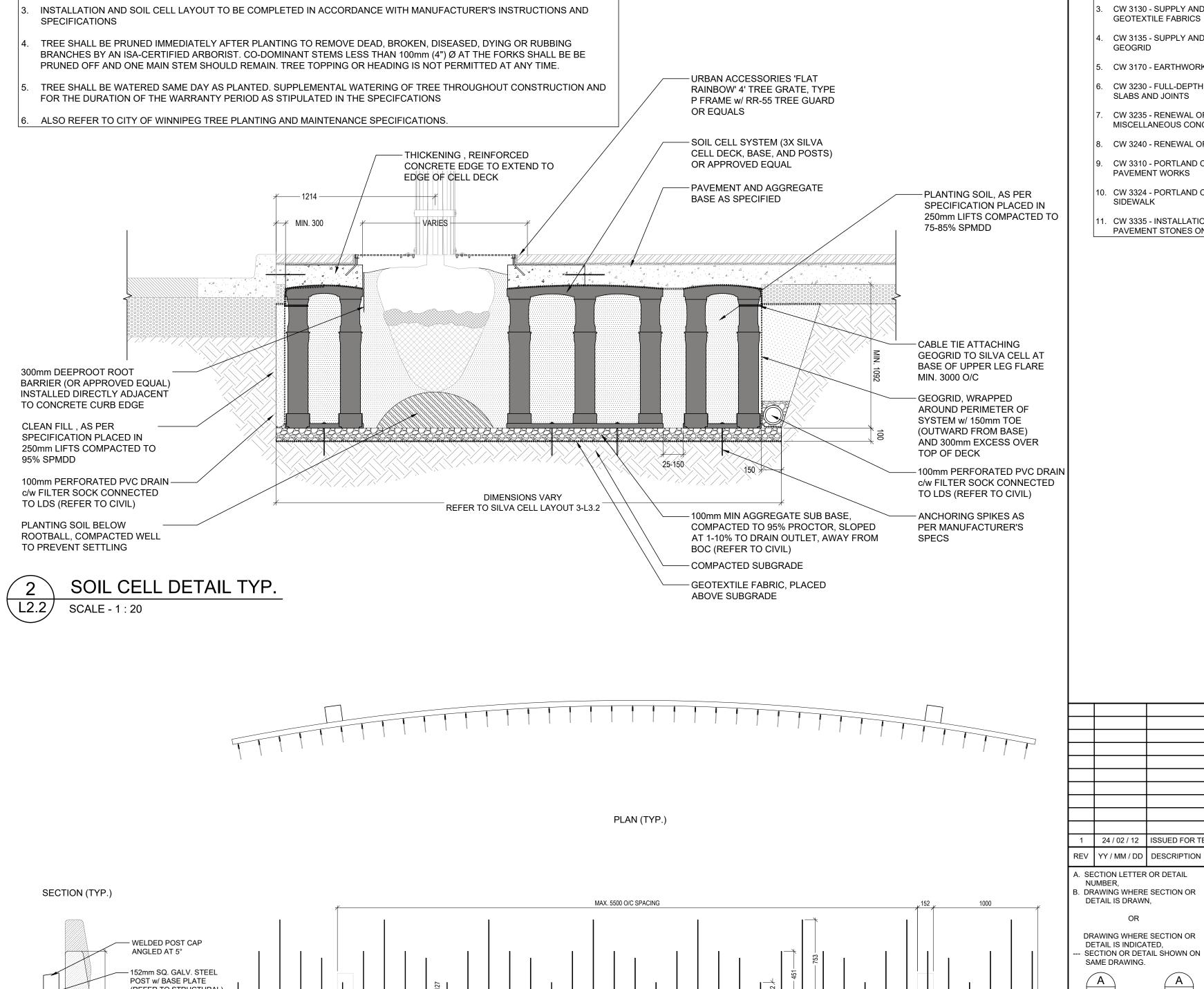
EXCAVATION FOR SOIL CELL SHALL BE MINIMUM OF 1200mm AND SHALL BE COMPLETE IN ACCORDANCE WITH ALL
