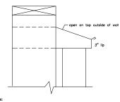
26 Gauge counter flashing complete with approx. 1/2" 45 degreee bottom kick out is to be installed over all membrane stripping. Terminate flashing about 1" above top of new roofing. Do not install any fasteners behind the cap flashing and use only lap joints. This is to allow easy removal for future repairs.
