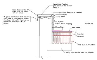
A continuous 18 gauge galvanized cleat is to be installed to insure outside face of flashing is firmly attached to outside face whenever outside face of flashing exceeds 3". No fasteners will be accepted on the outside face.
