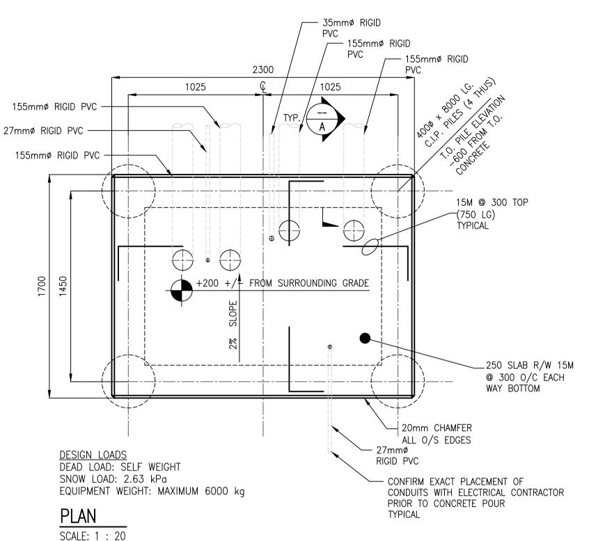
PLAN NOTES -PROVIDE 2 LAYERS 10 MIL POLYETHYLENE WRAPPED SONOTUBE GREASED COMPLETELY ON INSIDE FOR TOP 1800mm OF ALL PILES. -T.O.CONCRETE PAD ELEVATION TO BE SITE DETERMINED AND SHALL NOT BE LOWER THAN THE EXISTING TRANSFORMER PAD ELEVATION. USE 2% MINIMUM SLOPE AWAY FROM THE CONCRETE PAD FOR SURROUNDING GRADE. -SLAB SLEEVES SHALL BE LOCATED BETWEEN TOP AND/OR BOTTOM REINF.
