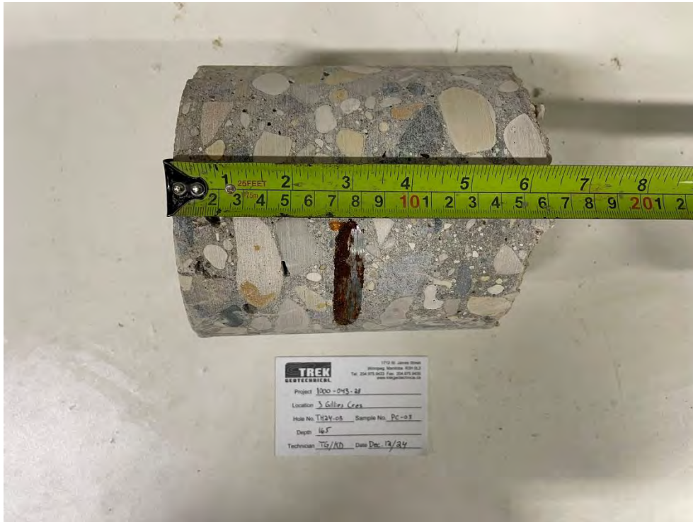
Photo 3: Pavement Core Sample at Test Hole TH24-03
