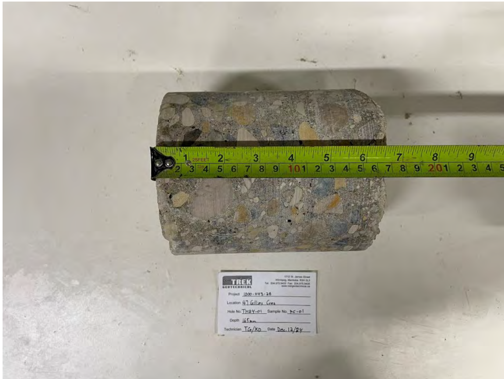
Photo 1: Pavement Core Sample at Test Hole TH24-01
