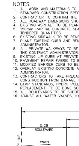
EXISTING BARRIER  $-\!\!\!/$ CURB TO BE RENEWED (DOWELLED, 100mm REVEAL) AS PER SD-205 (TYP.)
