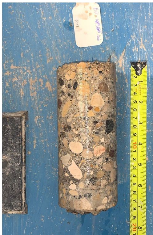
Figure 3 – Core Sample No. 166 - St. Anthony Ave
