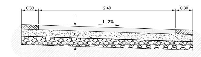
L75mm - TYPE MS1 ASPHALT (ONE LIFT) 125mm - 20mm GRANULAR B BASE COURSE MATERIAL GEOGRID - CLASS B 150mm - 50mm GRANULAR B SUB-BASE MATERIAL GEOTEXTILE FABRIC - SEPARATION/FILTRATION COMPACTED SUBGRADE
