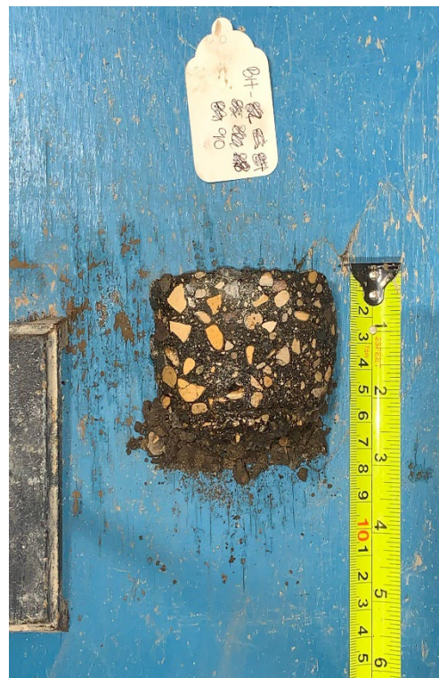
Figure 10 – Core Sample No. 90 – Middle Gate
