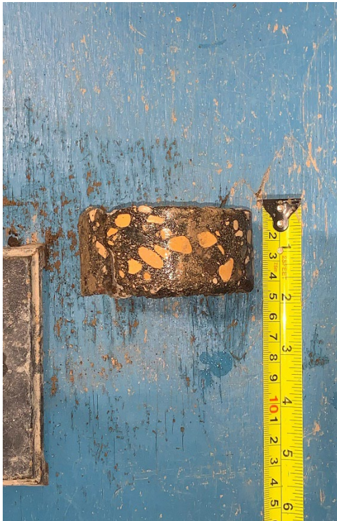
Figure 5 – Core Sample No. 85 – West Gate
