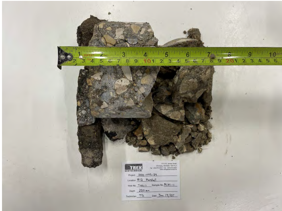
Photo 5: Pavement Core Sample at TH25-11
