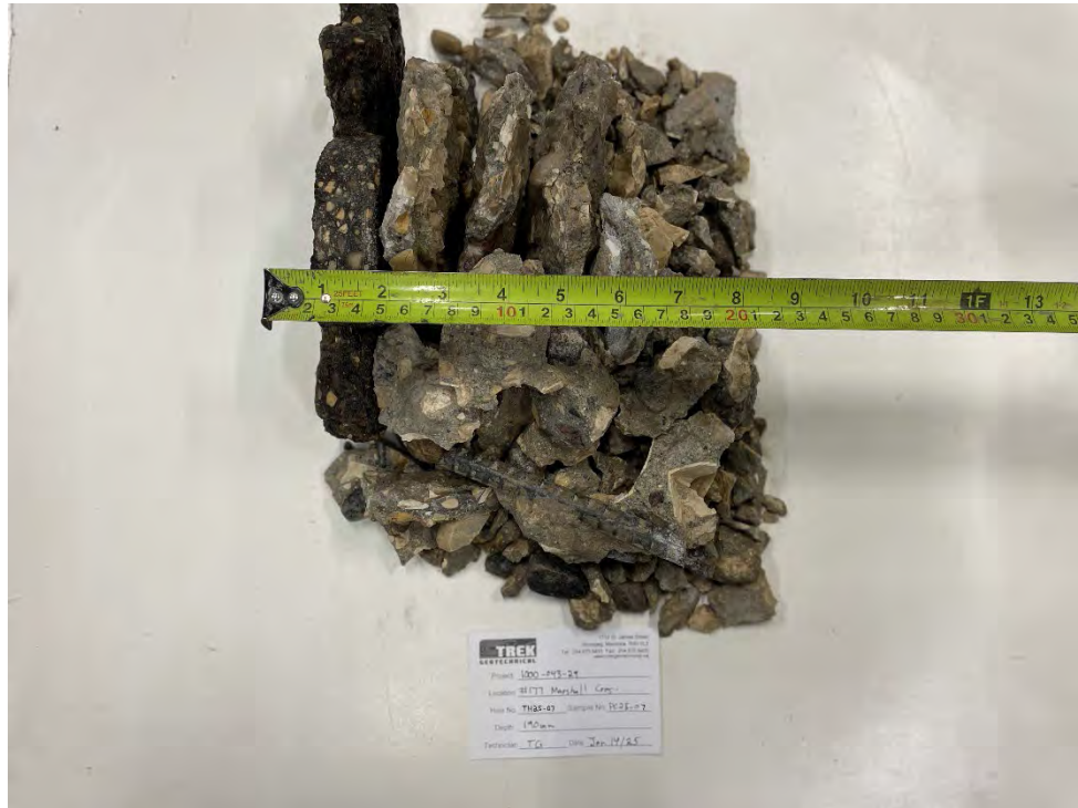
Photo 1: Pavement Core Sample at TH25-07
