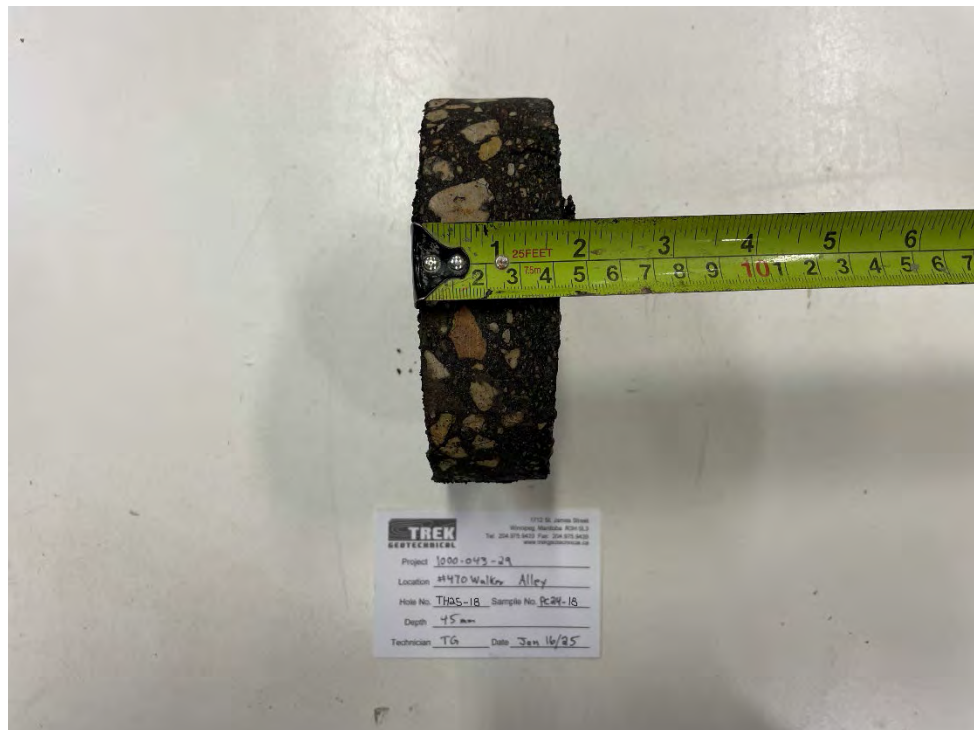
Photo 2: Pavement Core Sample at TH25-18
