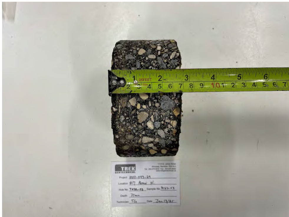
Photo 2: Pavement Core Sample at TH25-03
