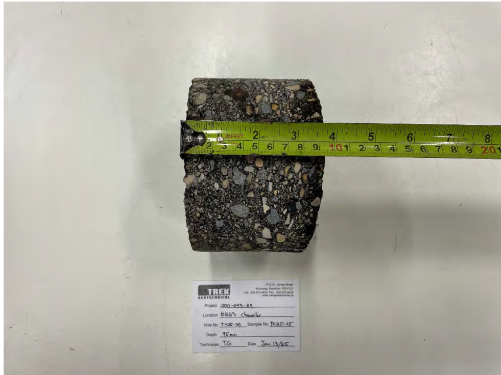
Photo 3: Pavement Core Sample at TH25-05
