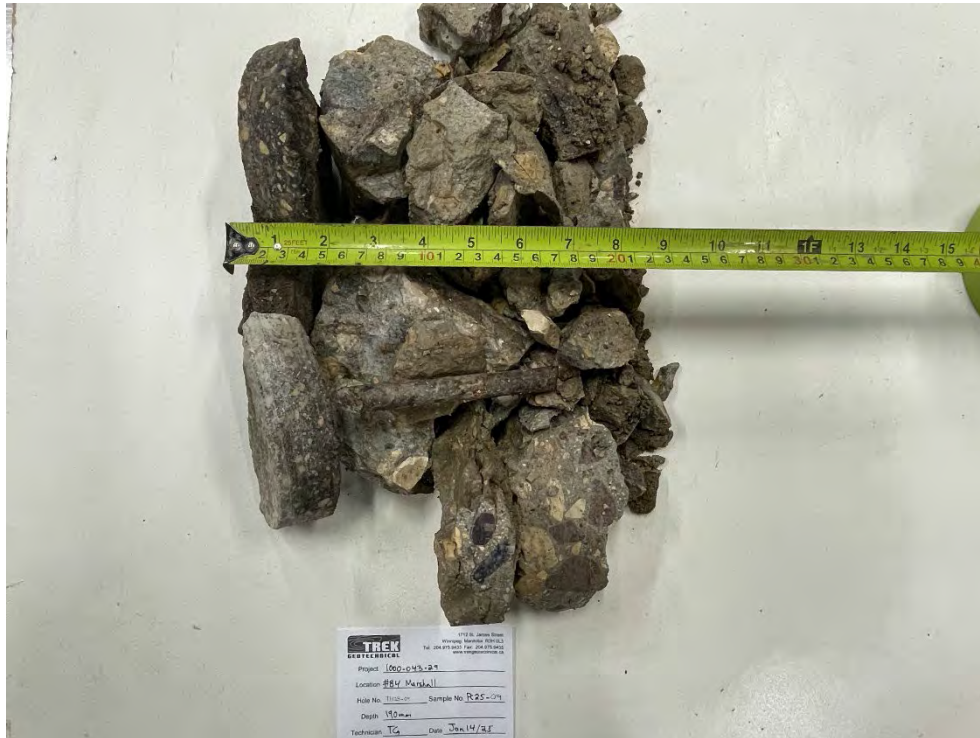
Photo 3: Pavement Core Sample at TH25-09
