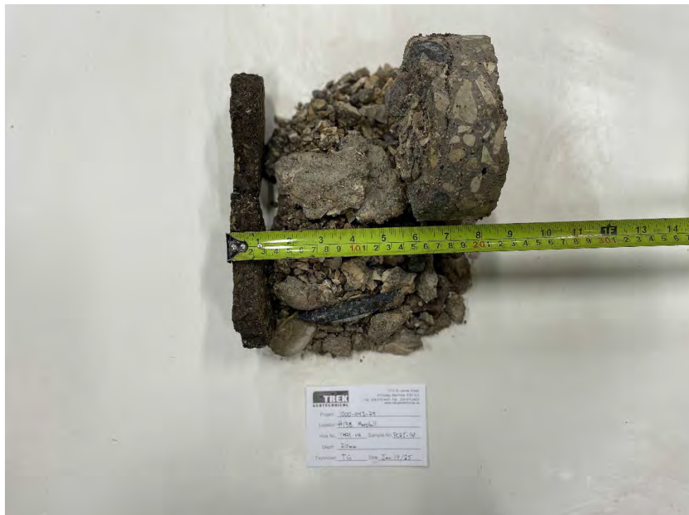
Photo 2: Pavement Core Sample at TH25-08
