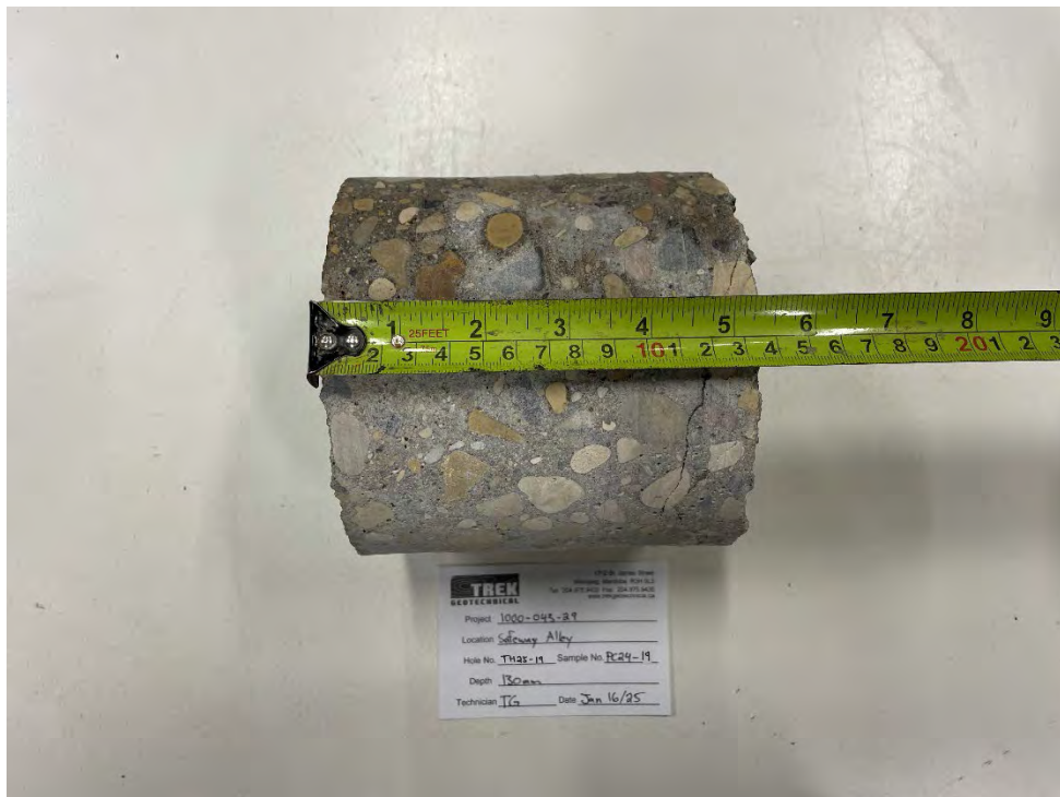
Photo 2: Pavement Core Sample at TH25-19
