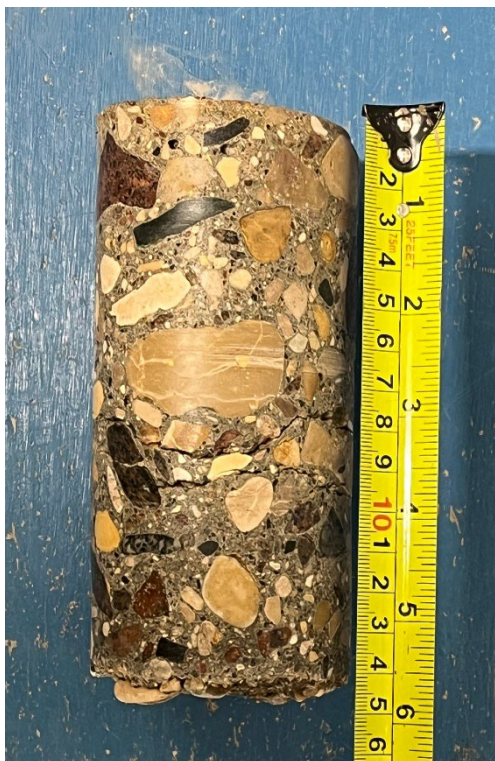
Figure 9 – Core Sample No. 227 – Callum Cr
