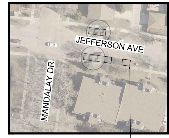
INSTALL 3.0x4.0 — 100mm REINFORCED CONCRETE PAD FOR NON—HEATED SHELTER
