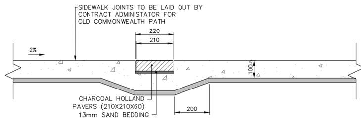
5 SIDEWALK WITH BLOCKOUT FOR PAVING STONE DETAIL
