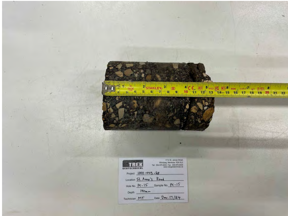
Photo 15: Pavement Core Sample at PC-15
