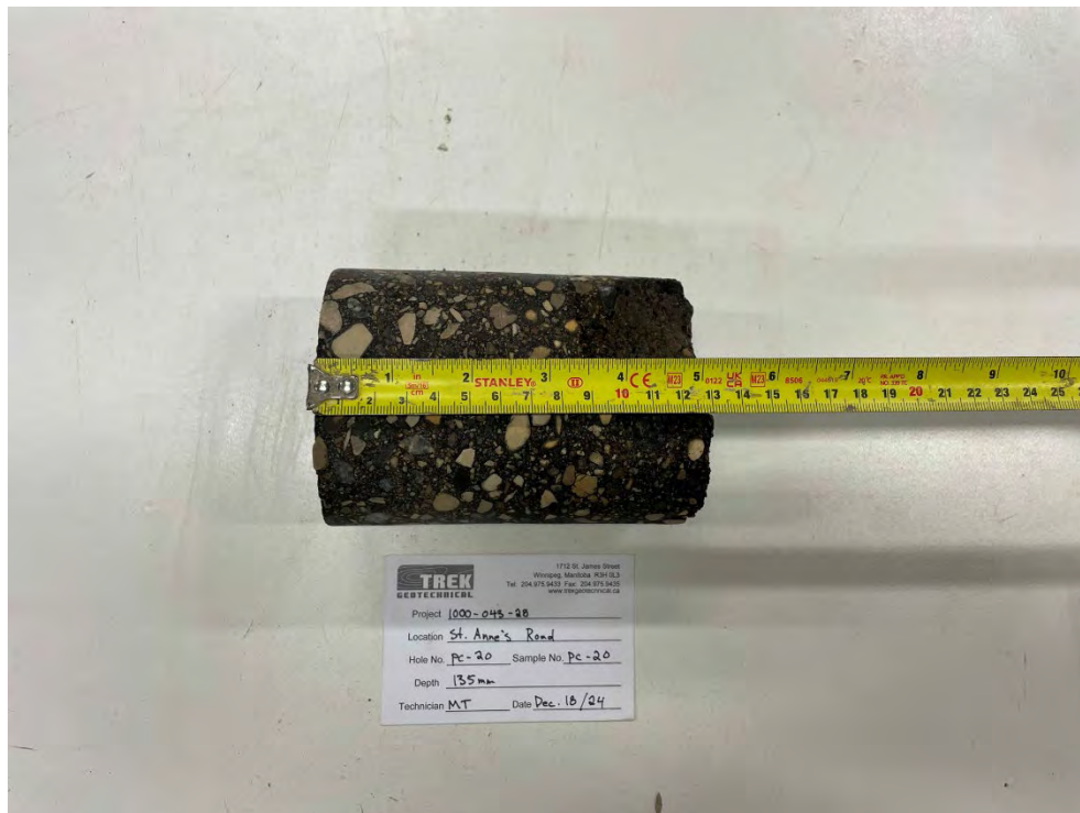
Photo 20: Pavement Core Sample at PC-20
