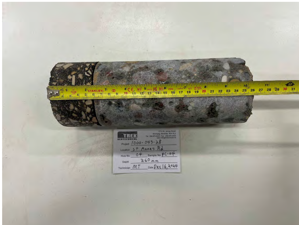
Photo 4: Pavement Core Sample at PC-04
