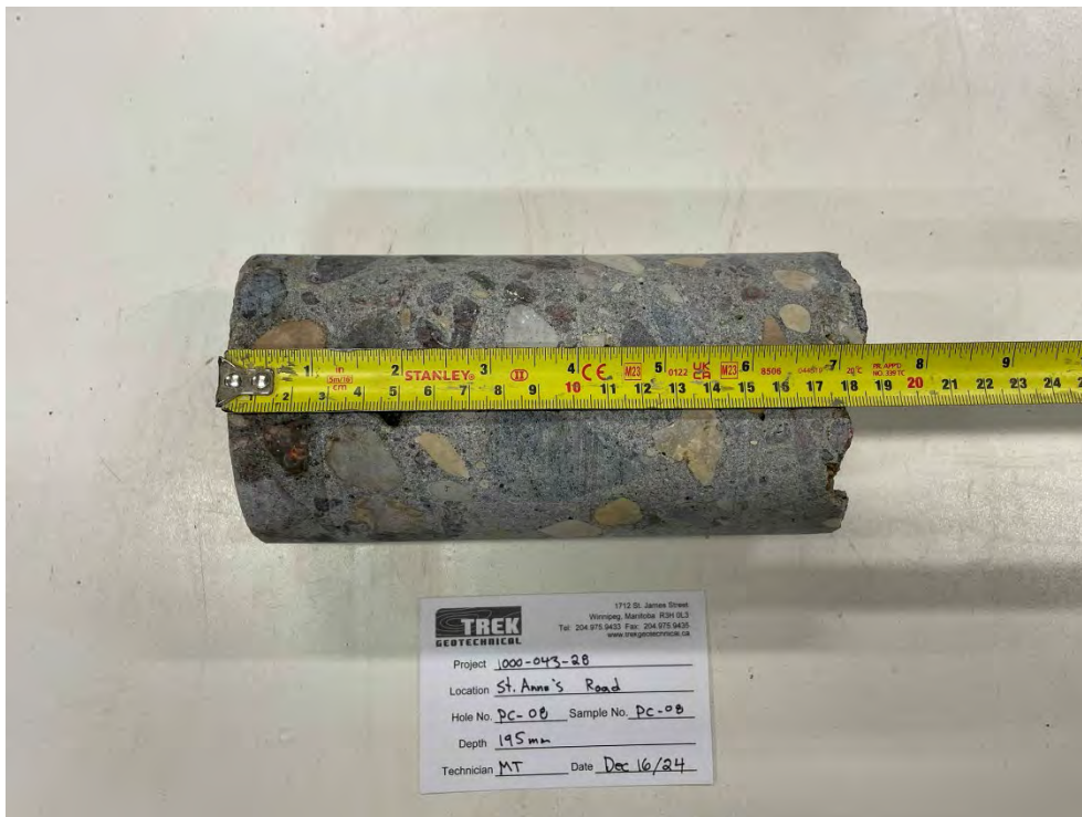
Photo 8: Pavement Core Sample at PC-08
