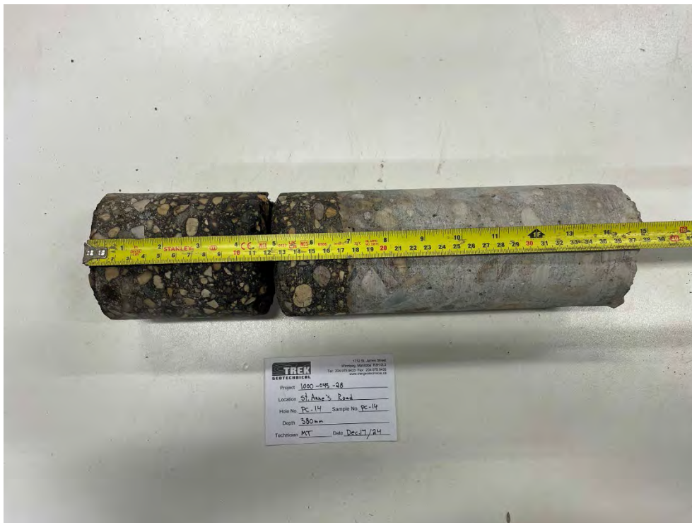
Photo 14: Pavement Core Sample at PC-14
