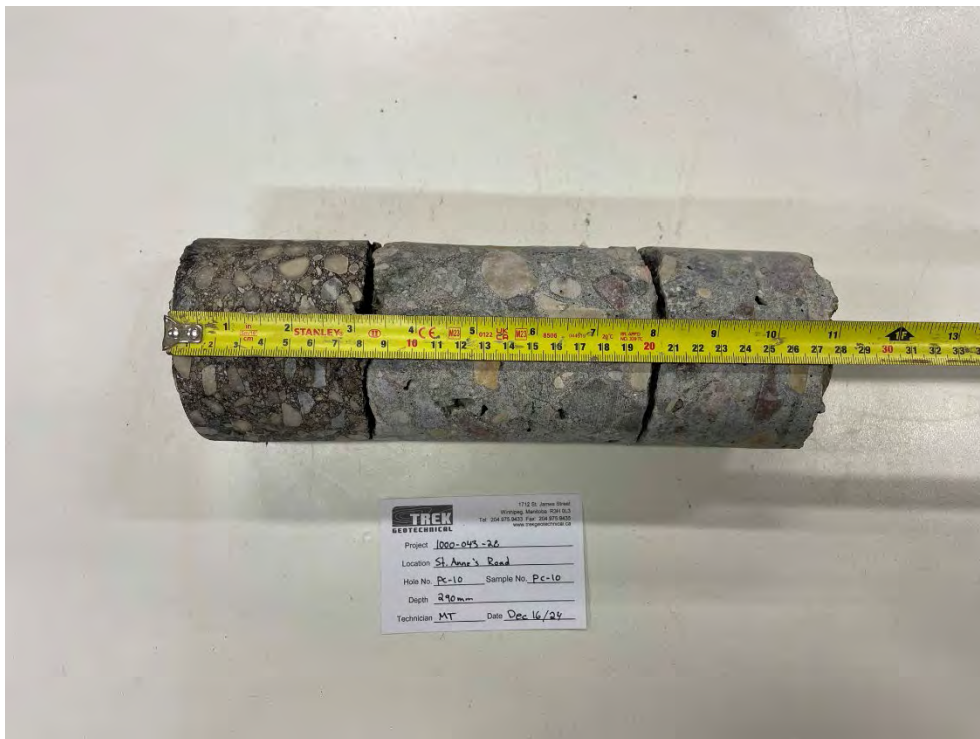
Photo 10: Pavement Core Sample at PC-10
