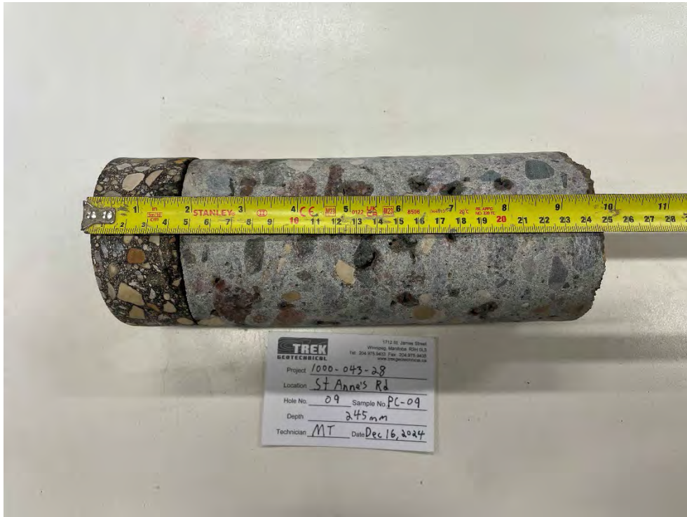
Photo 9: Pavement Core Sample at PC-09
