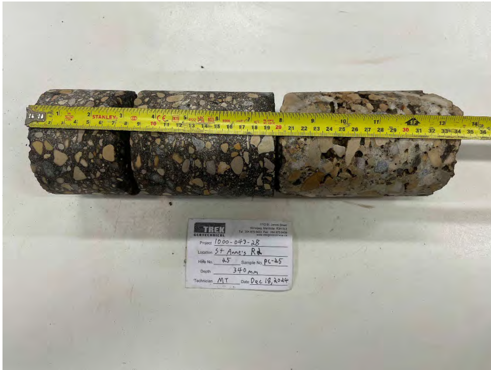
Photo 25: Pavement Core Sample at PC-25
