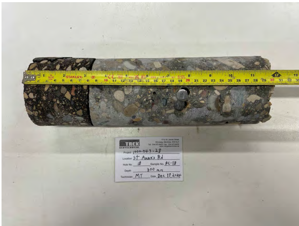
Photo 18: Pavement Core Sample at PC-18
