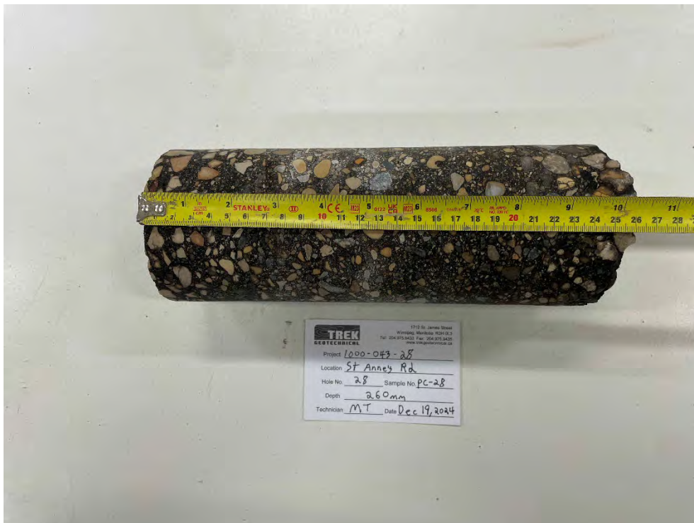
Photo 28: Pavement Core Sample at PC-28
