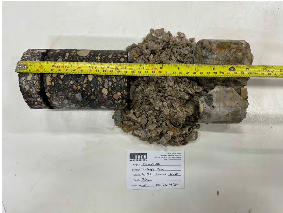
Photo 29: Pavement Core Sample at PC-29
