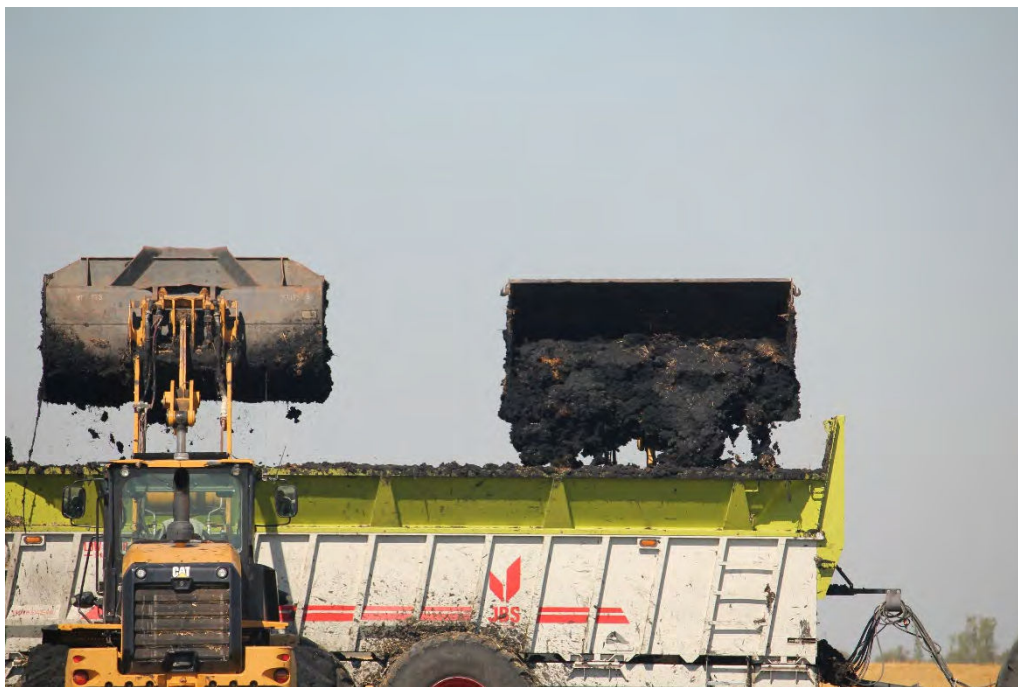
Photo 7: S1/2 29-12-01WPM – Loading Biosolids onto Spreader
