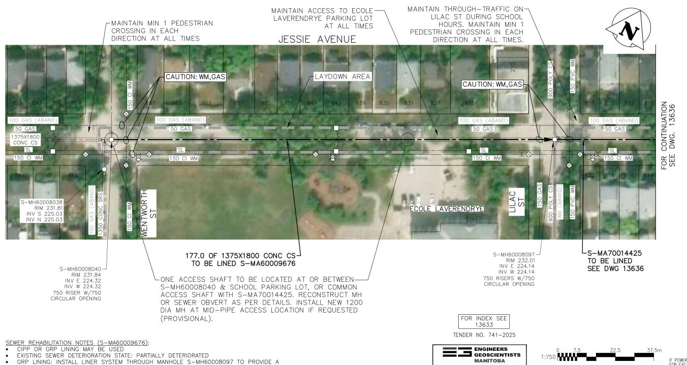
FROM SEWER VIDEO INSPECTION SEWER ID S-MA60009676 DISTANCE FROM MH ID S-MH60008040 DISTANCE DIAMETER CLOCK 12.8 1:00 150 26.0 150 11:00 27.5 150 2:00 27.5 150 10:00 150 42.2 2:00 42.2 150 10:00 57.9 150 10:00 61.8 150 10:00 73.1 150 3:00 73.1 150 9:00 79.2 150 10:00 88.7 150 2:00 88.7 150 10:00 92.1 150 3:00 92.1 150 9:00 103.9 150 2:00 150 103.9 10:00
