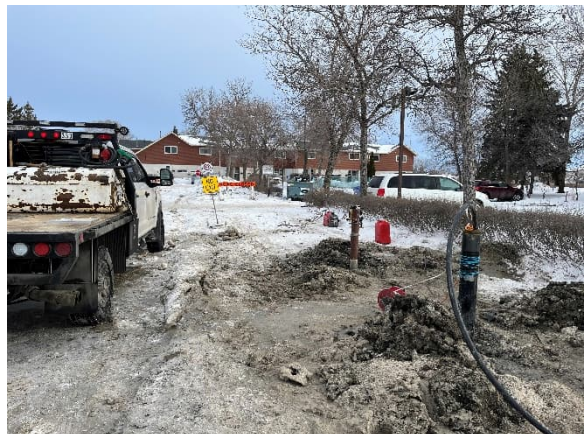
Photo 10: View of MW26-LM-01 (red protective cover) and PW26-LM-01 (black steel stick-up)
