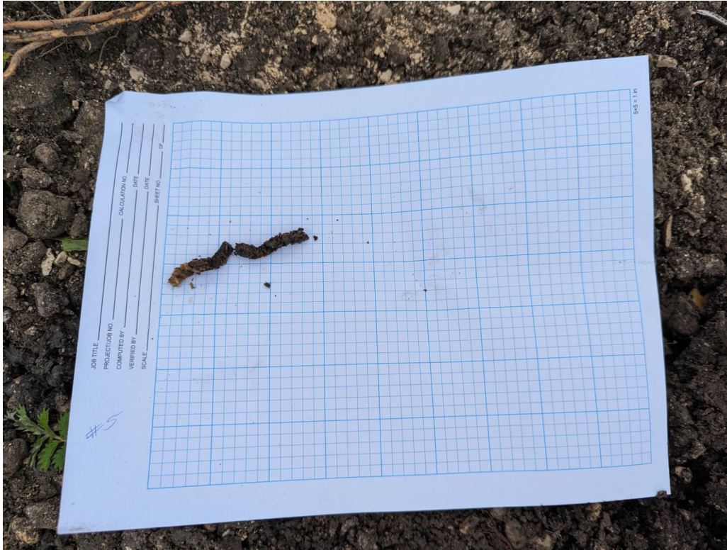
Photograph 45 Core sample obtained from pile at Test Pit No. 2. Note: Rotten.
