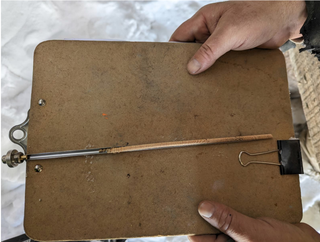
Photograph 39 Typical core sample obtained from Piles C1/D1. Note: No rot detected.
