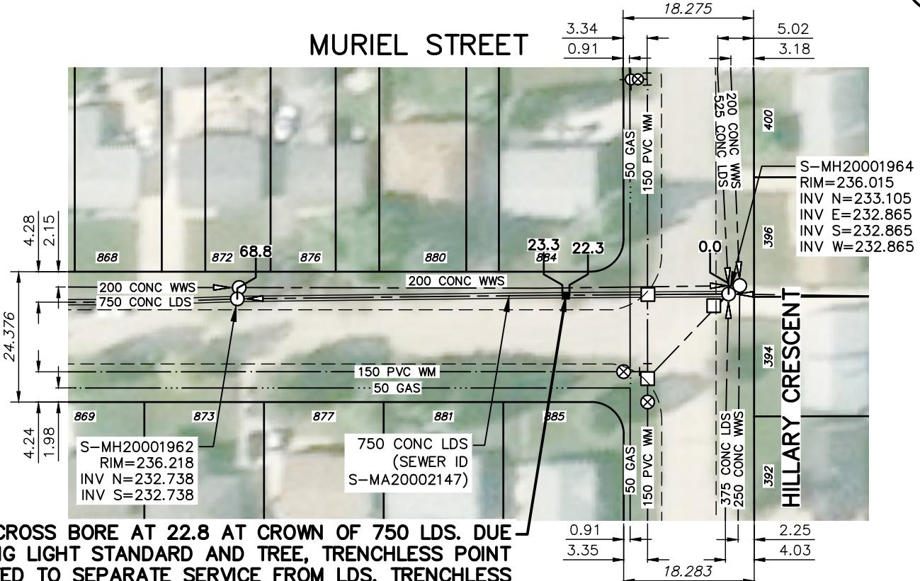
EXISTING SEWER SERVICE CROSS BORE AT 22.8 AT CROWN OF 750 LDS. DUE TO PROXIMITY TO EXISTING LIGHT STANDARD AND TREE, TRENCHLESS POINT REPAIR TO BE COMPLETED TO SEPARATE SERVICE FROM LDS. TRENCHLESS POINT REPAIR TO EXTEND MIN. 0.5m ON EACH SIDE OF C/L OF CROSS BORE.
