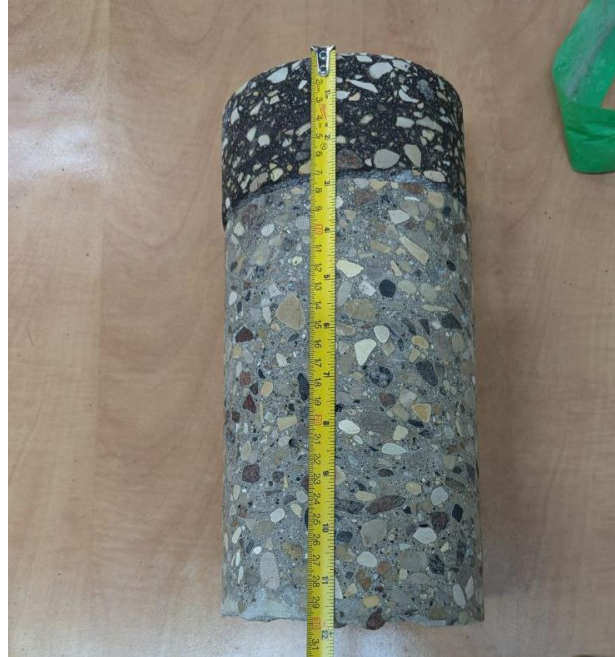
, Core 2 (Asphalt Thk 70mm, Concrete Thk 230mm)
