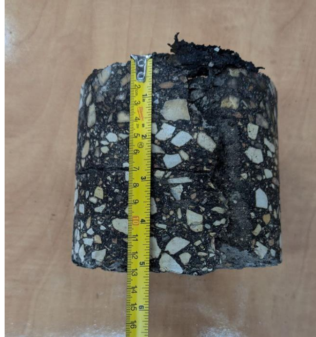
Core 2B (Asphalt Thk 130mm)
