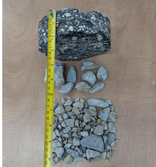
Core 6 (Asphalt Thk 50mm, Concrete 170 Thk mm)
