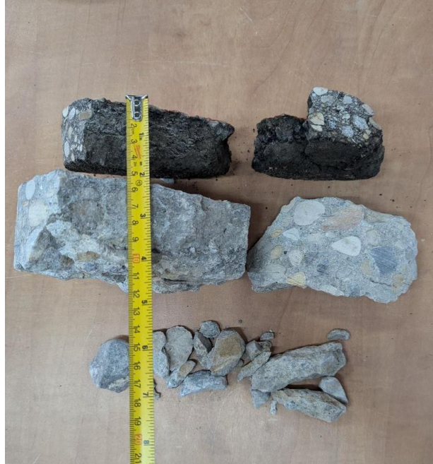
Core 17 (Asphalt Thk 40mm, Conc Thk 140mm)
