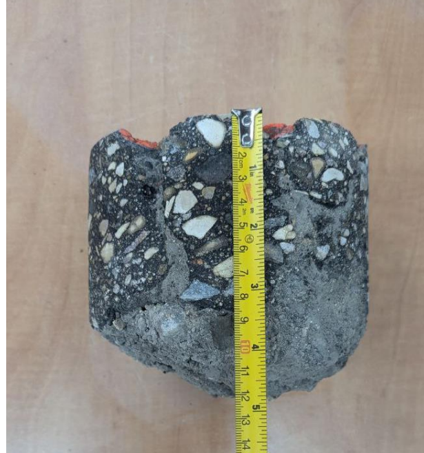
Core 15 (Asphalt Thk 90mm, Conc Thk 140mm)
