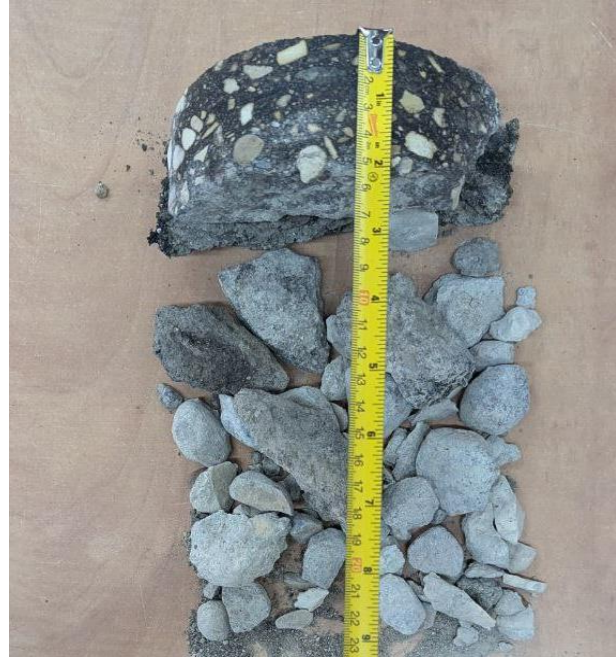
Core 12 (Asphalt Thk 50mm, Conc Thk 140mm)
