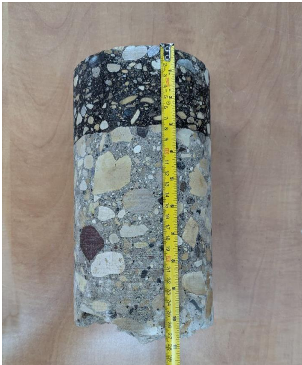
Core 7 (Asphalt Thk 75mm, Conc Thk 190mm)
