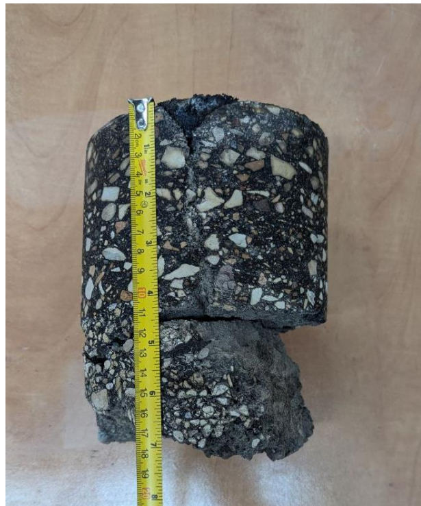
, Core 2A (Asphalt Thk 180mm)
