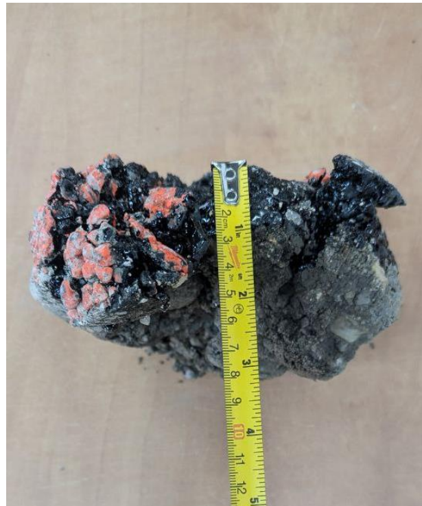
Core 16 (Asphalt Thk 60mm, Conc Thk 100mm)
