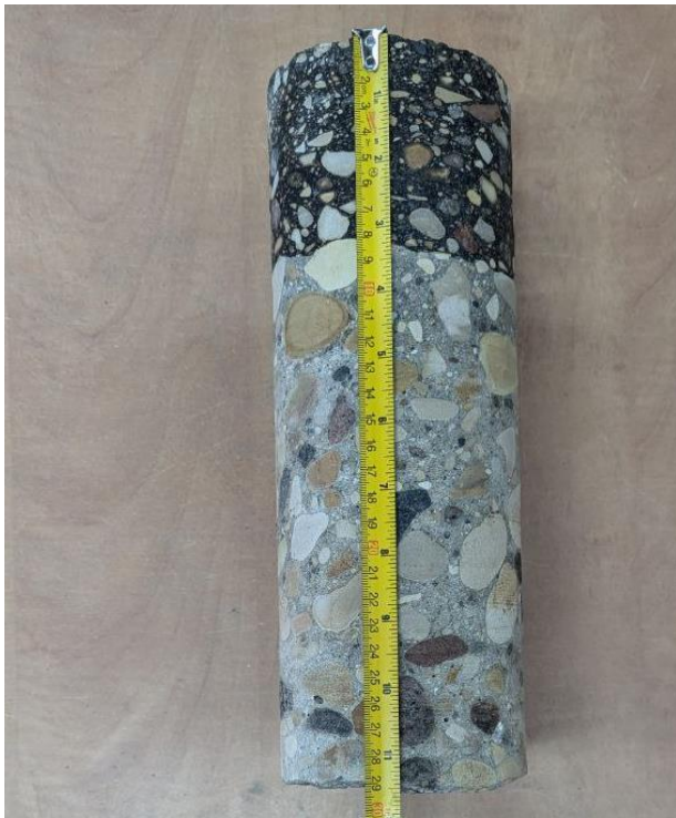
Core 13 (Asphalt Thk 85mm, Conc Thk 210mm)
