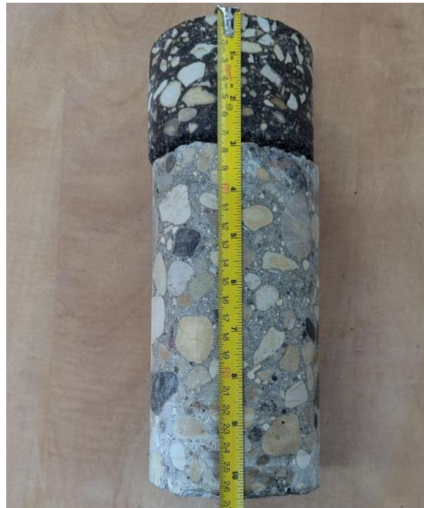
Core 14 (Asphalt Thk 70mm, Conc Thk 190mm)
