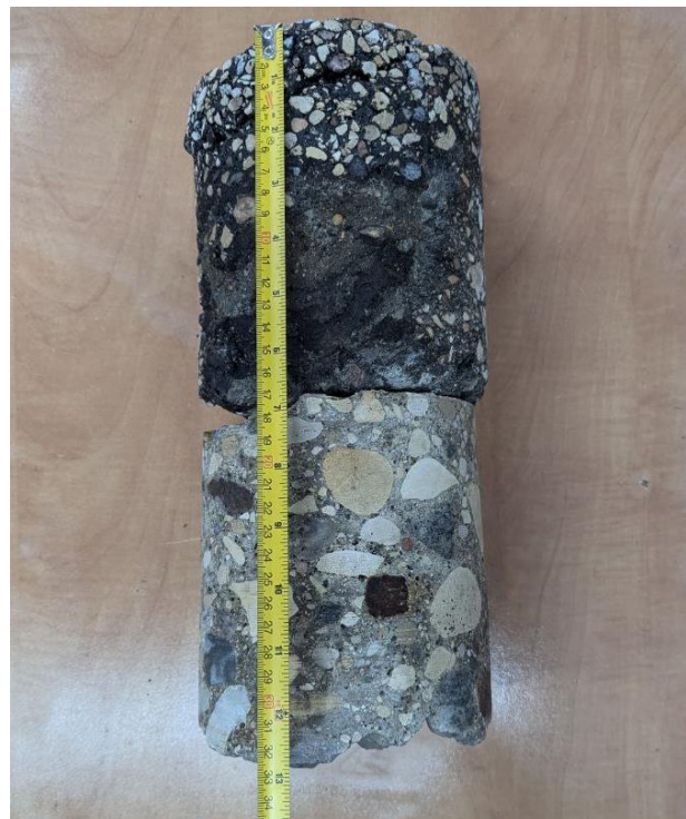
Core 4 (Asphalt Thk 170mm, Conc Thk 170mm)
