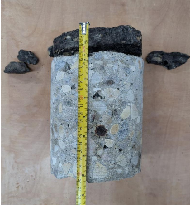
Core 5 (Asphalt Thk 35mm, Conc Thk 180mm)
