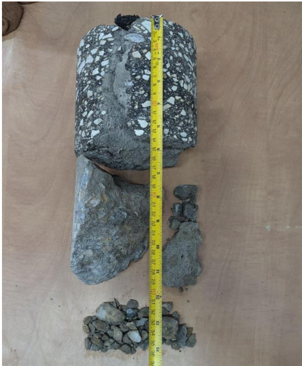
Core 3 (Asphalt Thk 140mm, Conc Thk 230mm)
