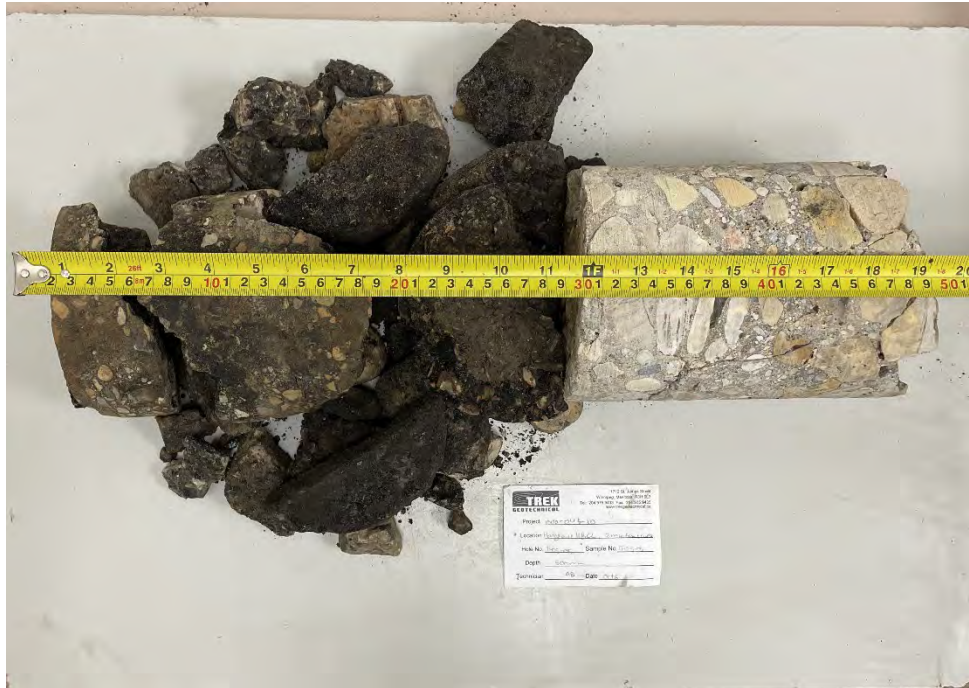
Photo 1: Pavement Core Sample at TH25-05
