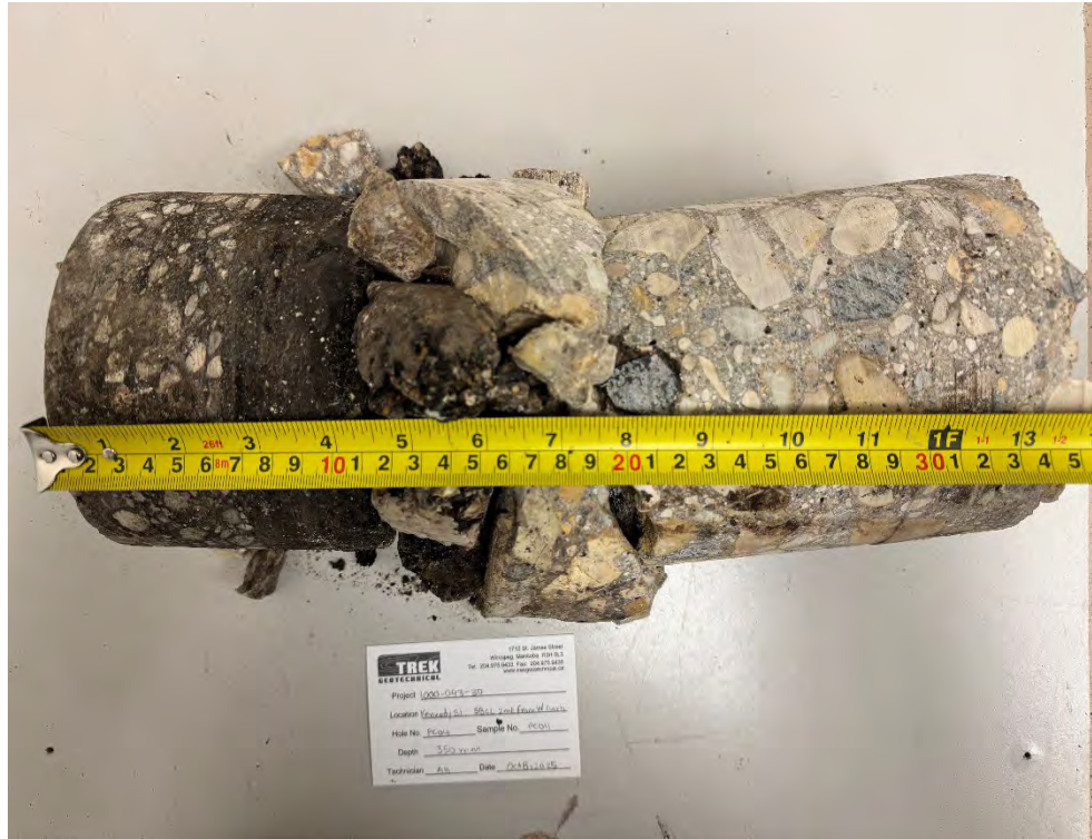
Photo 3: Pavement Core Sample at PC25-04
