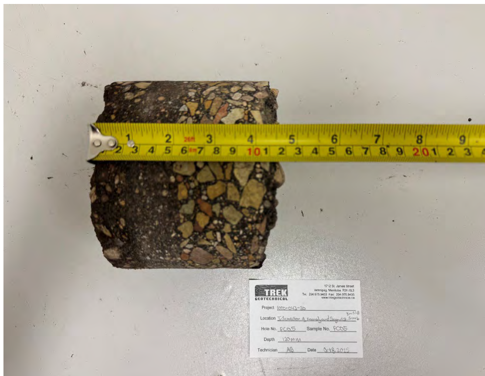
Photo 3: Pavement Core Sample at PC25-04
