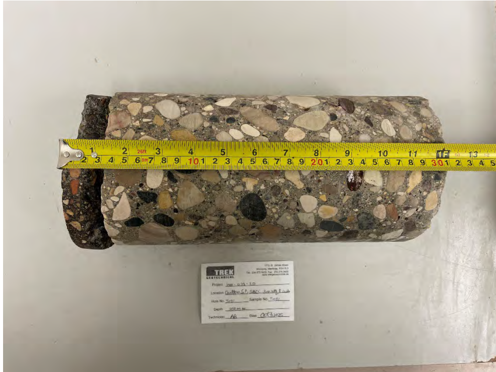
Photo 1: Pavement Core Sample at TH25-01
