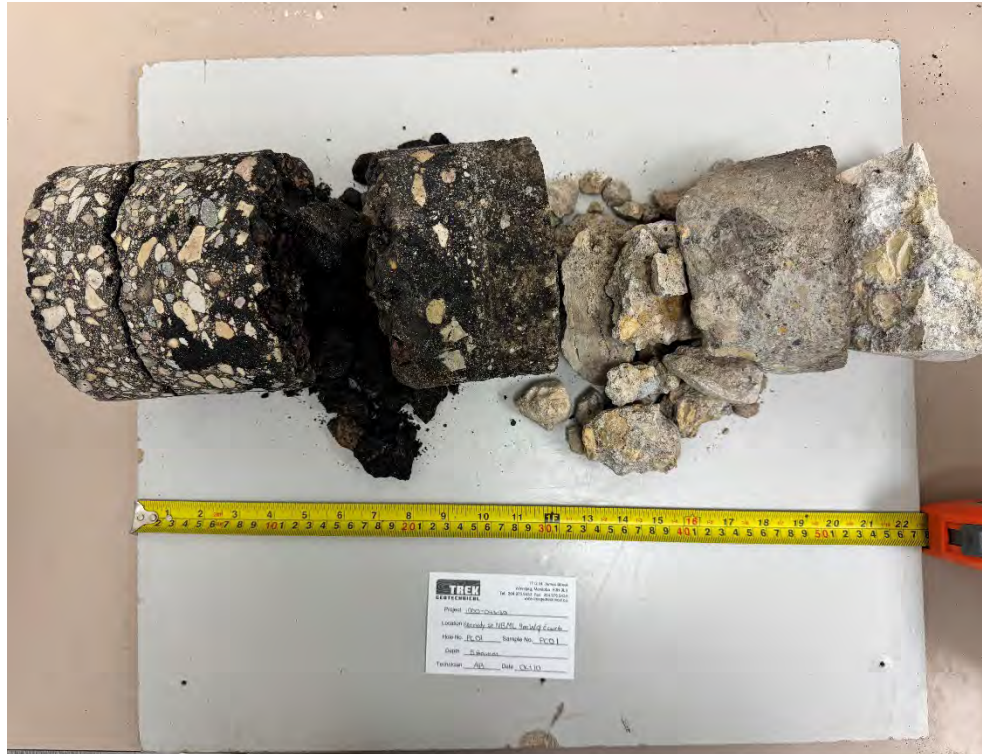
Photo 1: Pavement Core Sample at PC25-01
