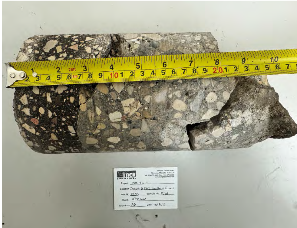
Photo 1: Pavement Core Sample at PC25-03
