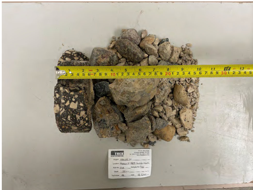
Photo 1: Pavement Core Sample at TH25-05
