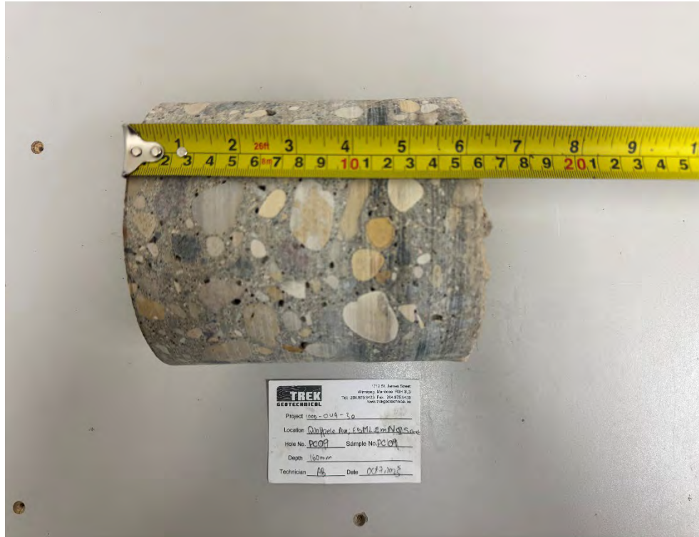
Photo 3: Pavement Core Sample at PC25-09
