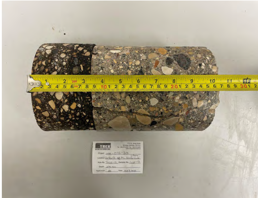
Photo 1: Pavement Core Sample at TH25-12
