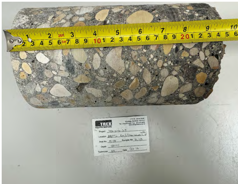
Photo 1: Pavement Core Sample at PC25-27
