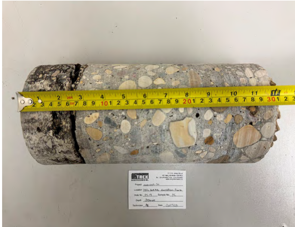
Photo 1: Pavement Core Sample at PC25-19
