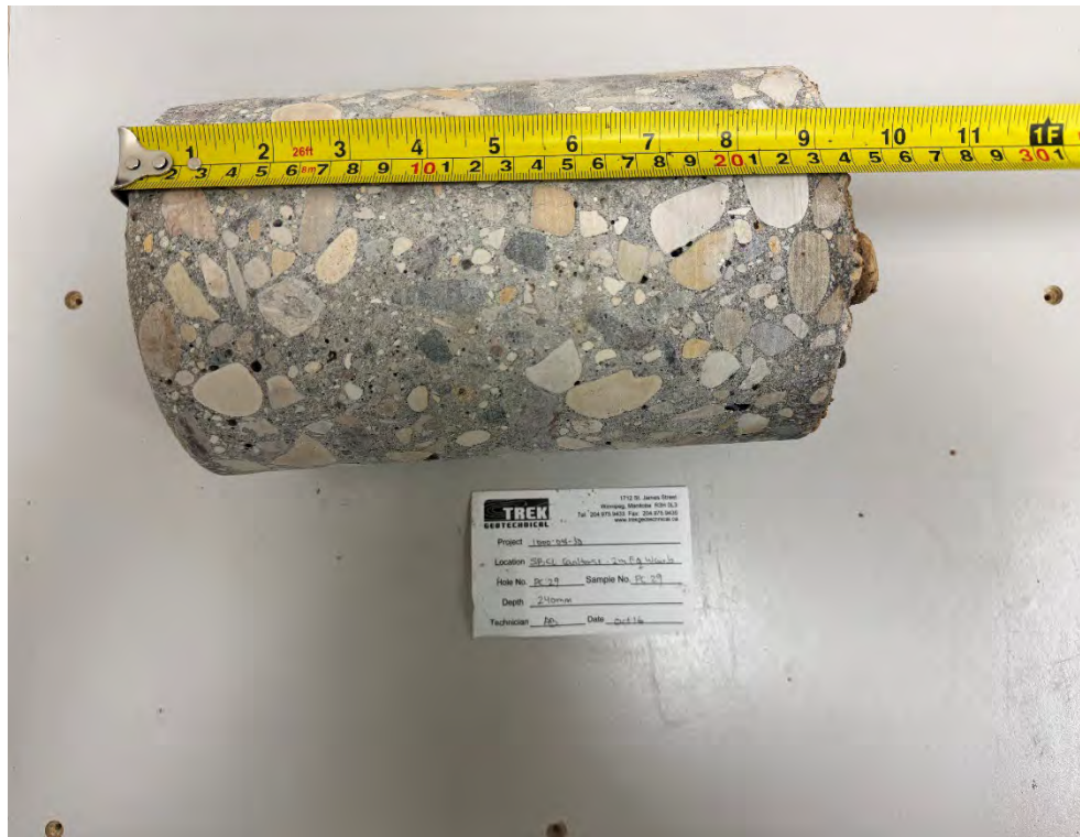
Photo 3: Pavement Core Sample at PC25-29
