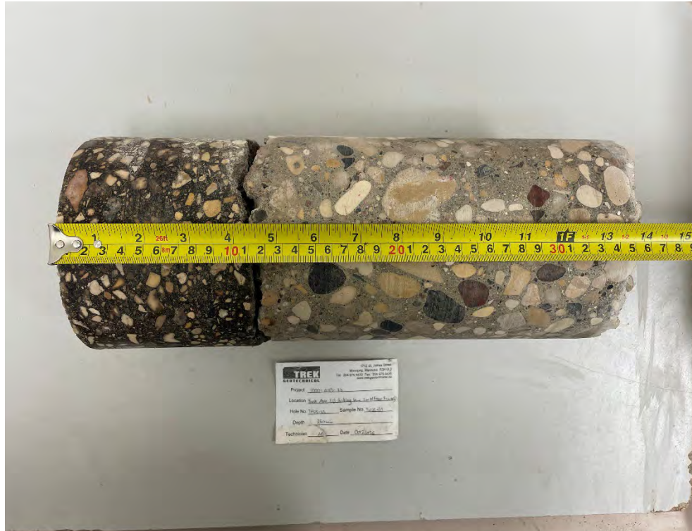
Photo 1: Pavement Core Sample at TH25-33
