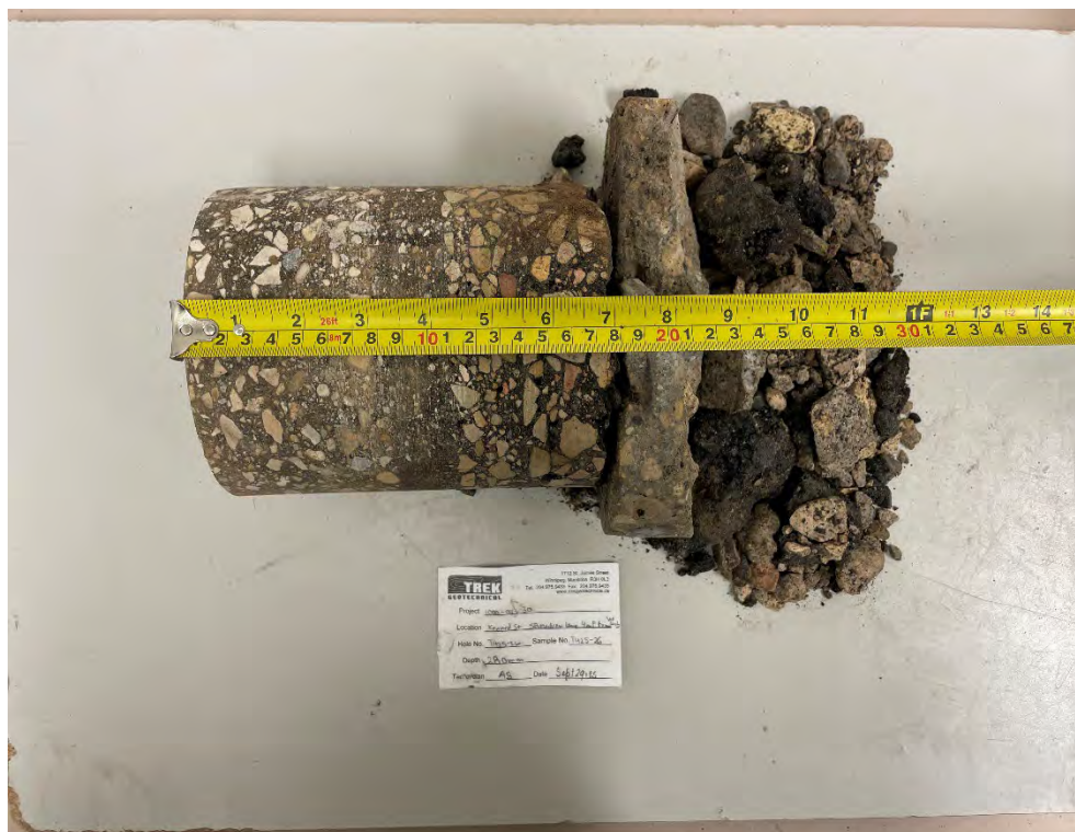
Photo 3: Pavement Core Sample at TH25-25
