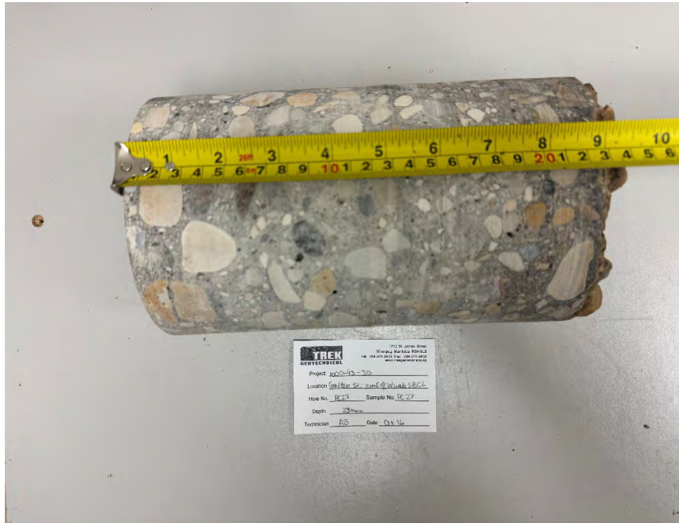
Photo 1: Pavement Core Sample at PC25-27
