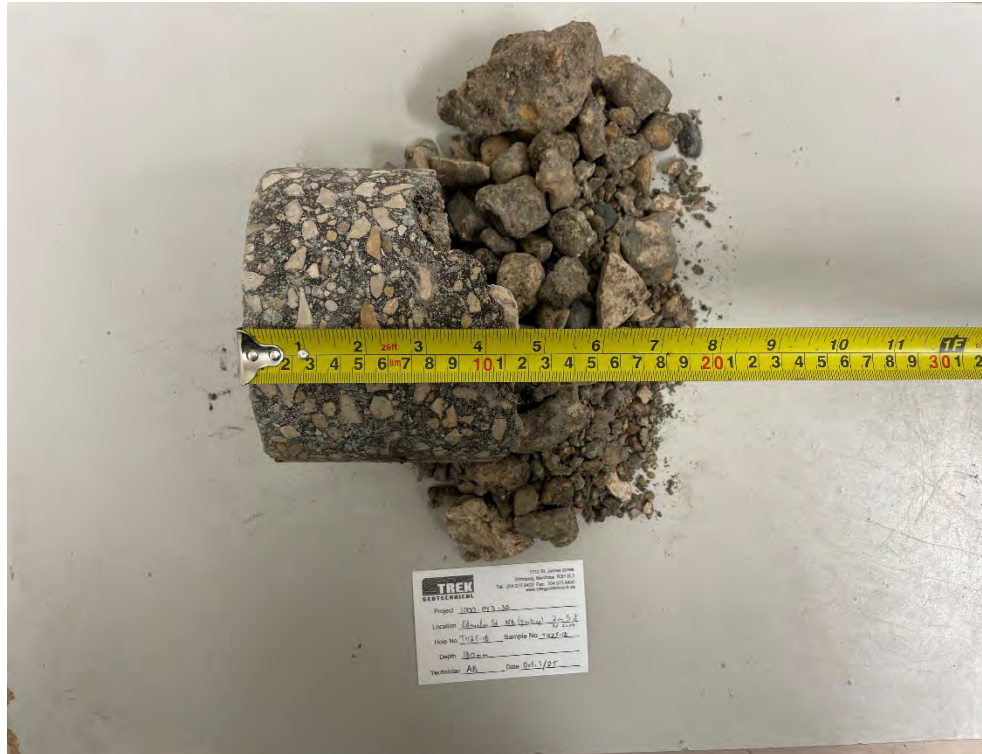
Photo 1: Pavement Core Sample at TH25-18
