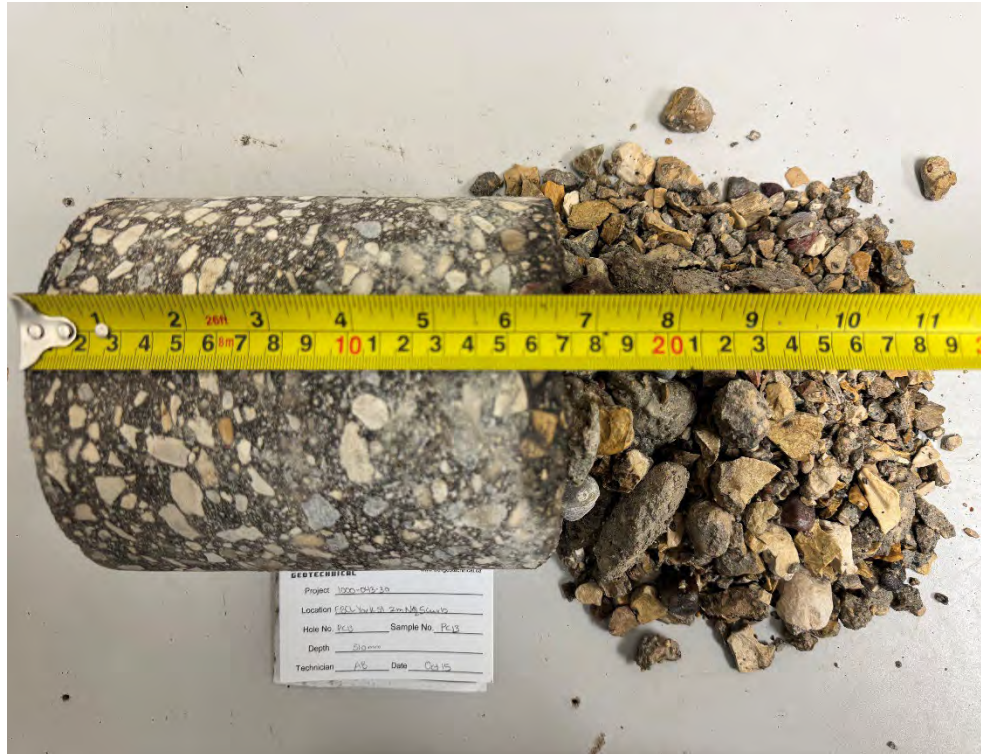
Photo 1: Pavement Core Sample at PC25-13
