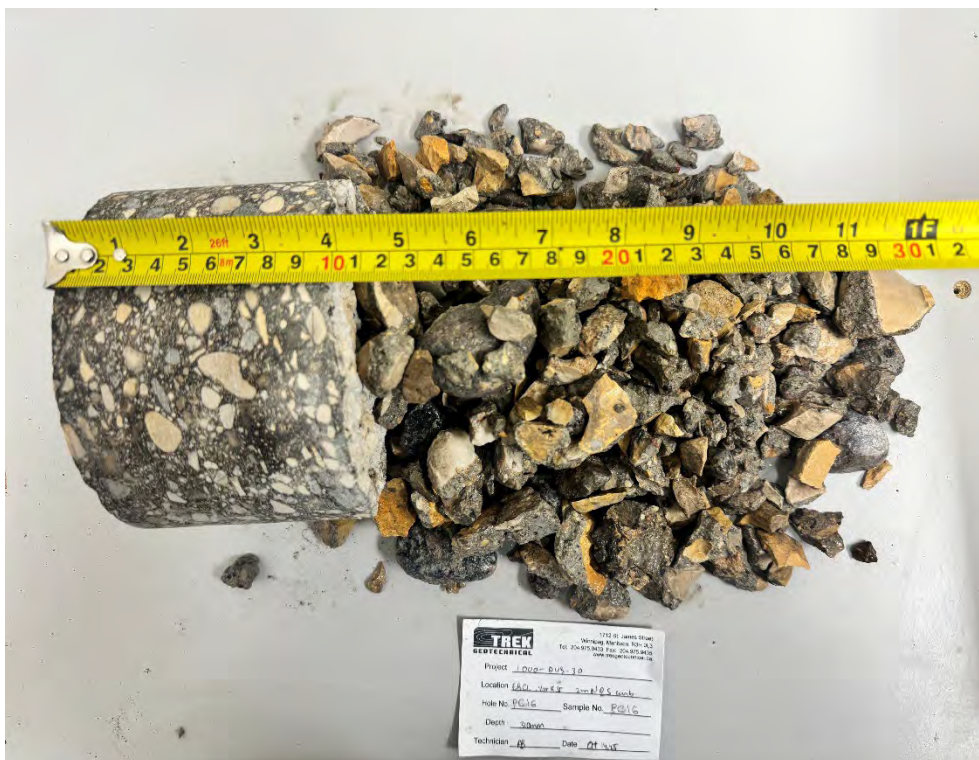
Photo 3: Pavement Core Sample at PC25-15
