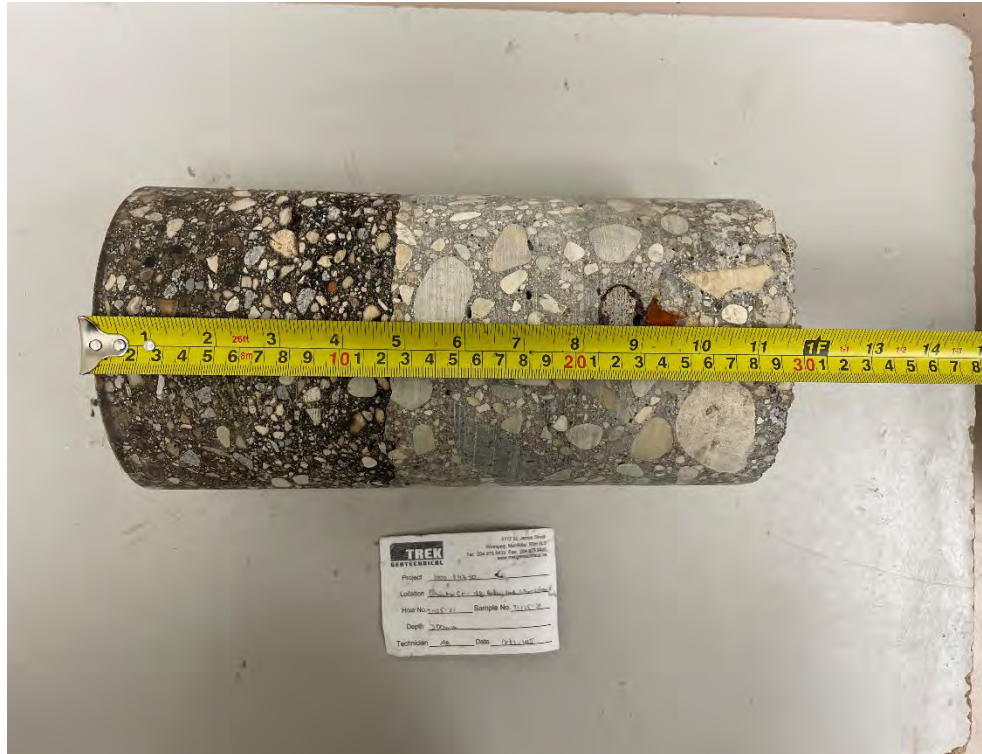
Photo 3: Pavement Core Sample at TH25-21
