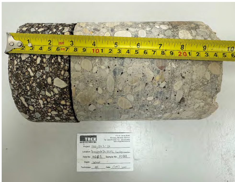
Photo 1: Pavement Core Sample at PC25-03
