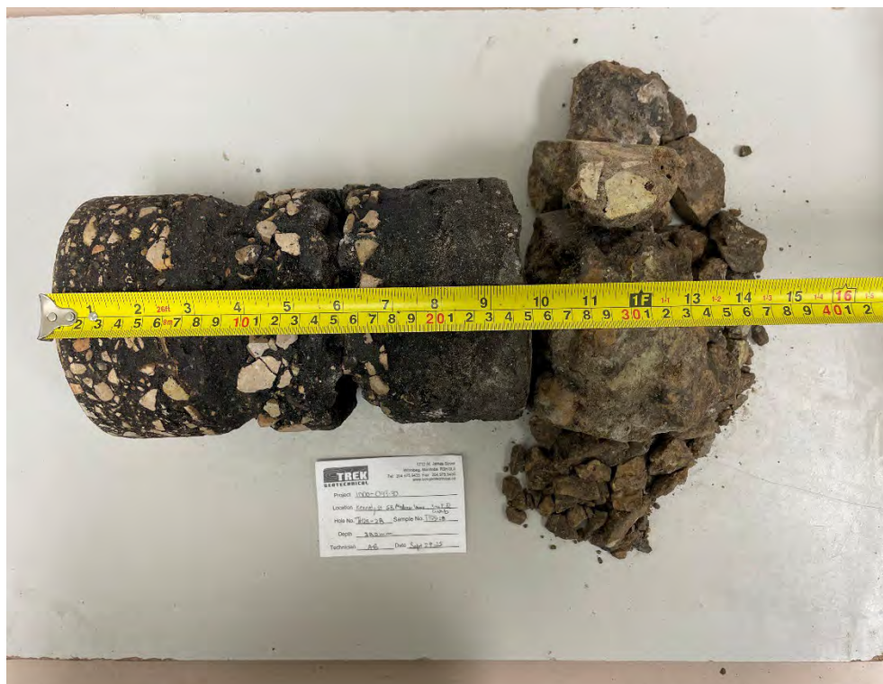
Photo 5: Pavement Core Sample at TH25-27
