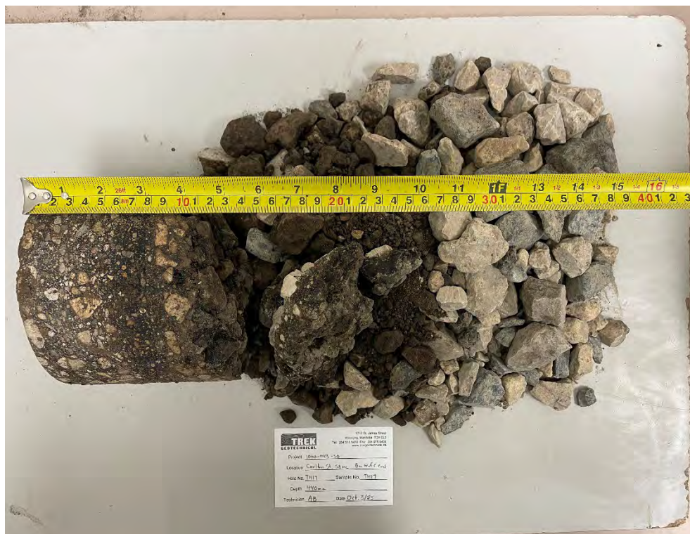
Photo 5: Pavement Core Sample at TH25-16
