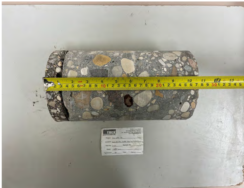
Photo 1: Pavement Core Sample at TH25-33
