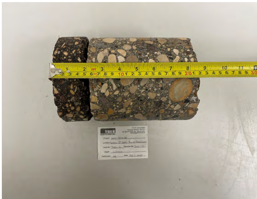
Photo 1: Pavement Core Sample at TH25-12
