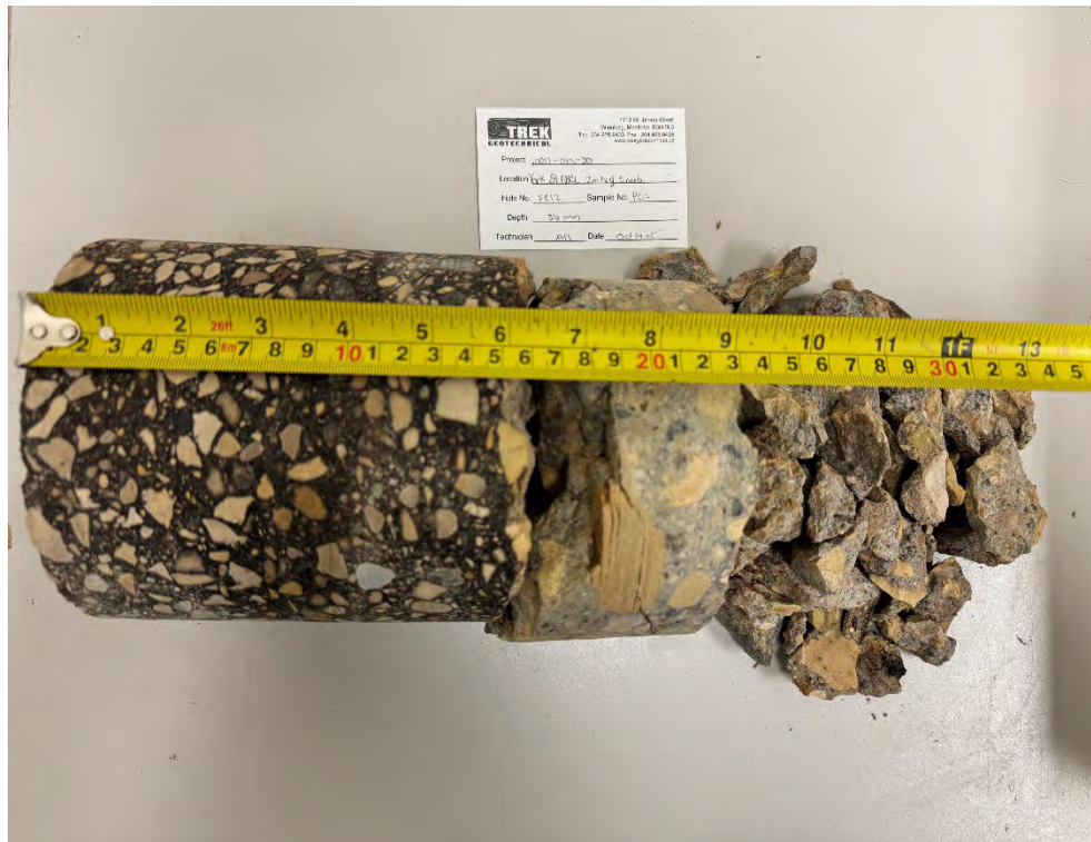
Photo 5: Pavement Core Sample at PC25-17
