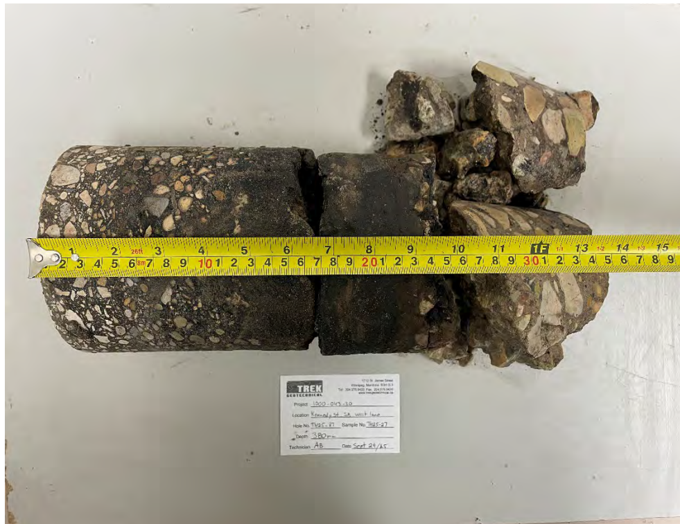
Photo 5: Pavement Core Sample at TH25-27
