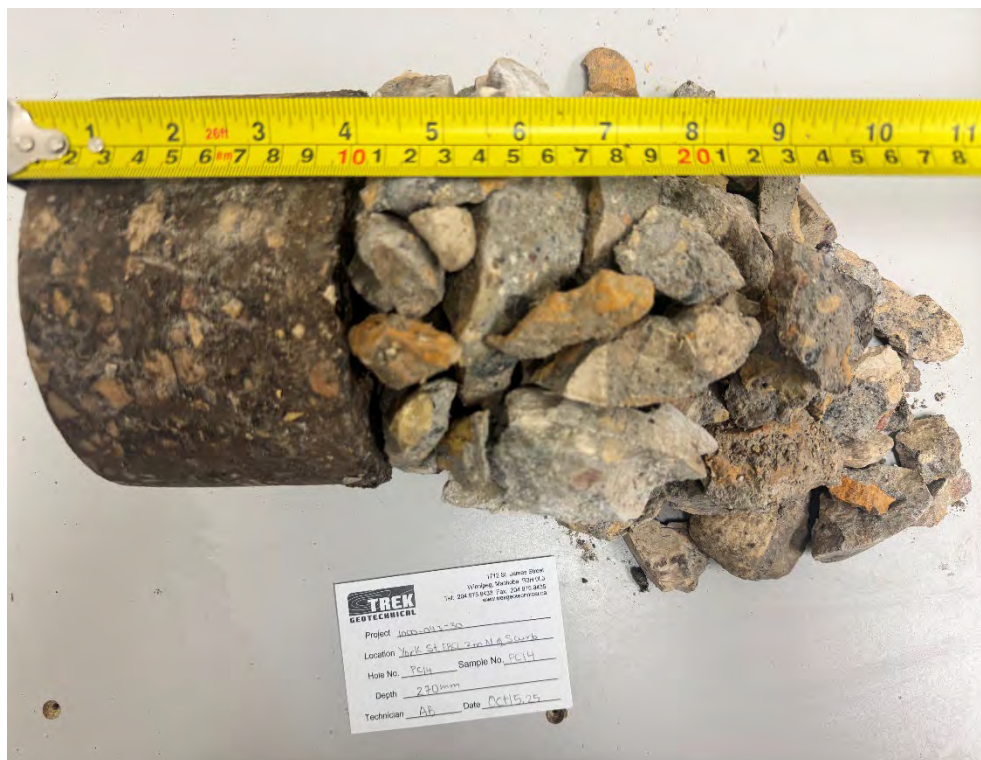
Photo 1: Pavement Core Sample at PC25-13
