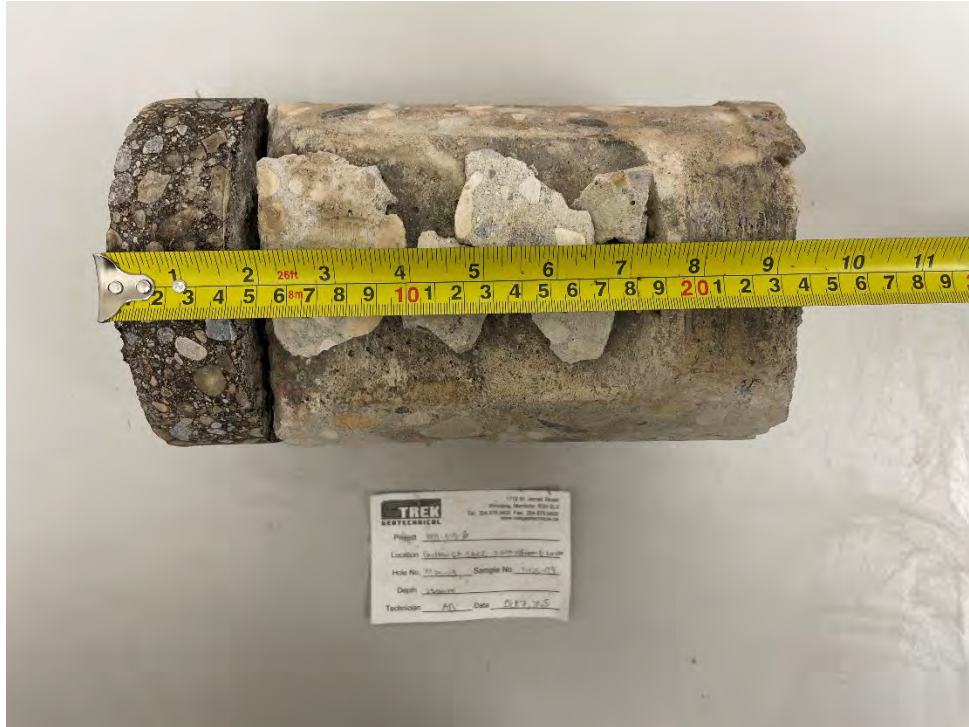
Photo 3: Pavement Core Sample at TH25-03
