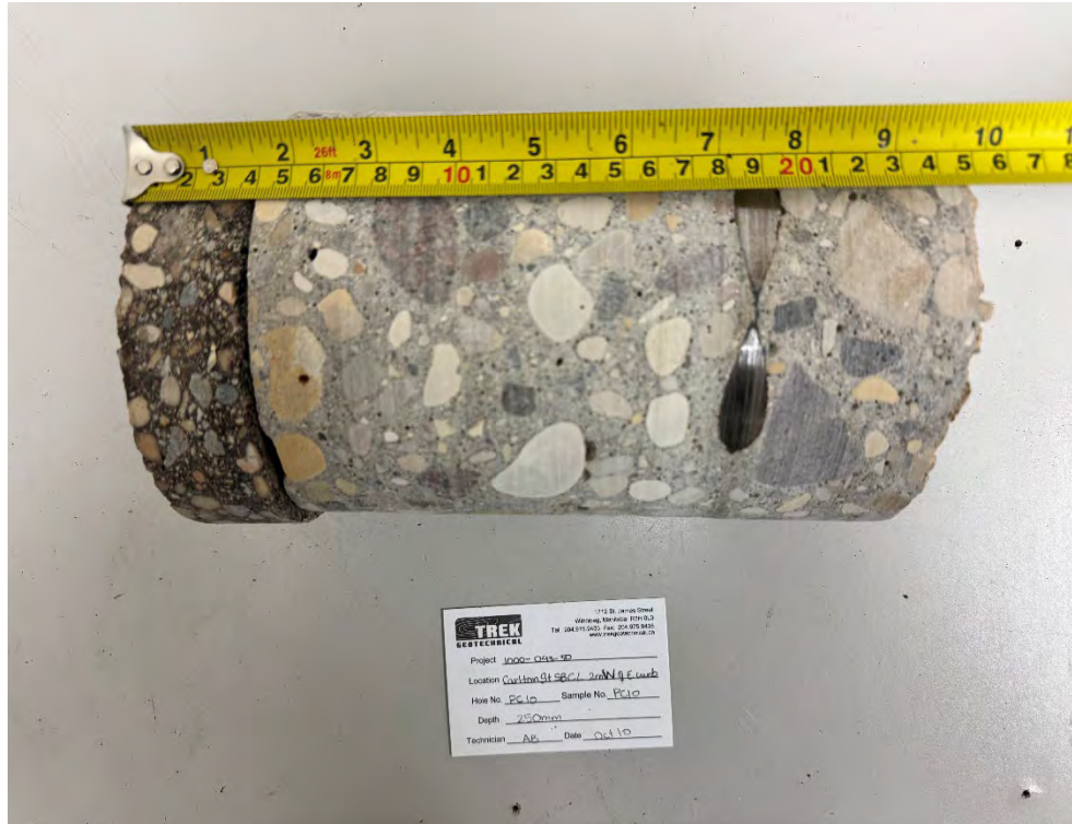
Photo 1: Pavement Core Sample at PC25-10
