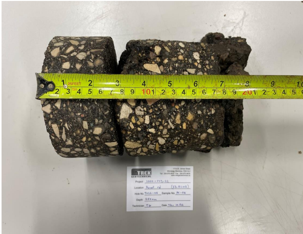
Photo 4: Pavement Core Sample at TH22-06
