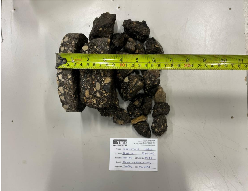
Photo 3: Pavement Core Sample at TH22-08
