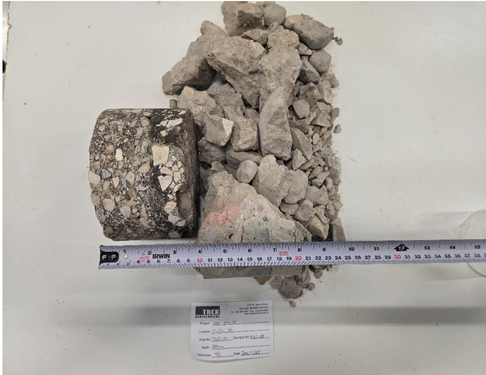
Photo 3: Pavement Core Sample at TH25-10
