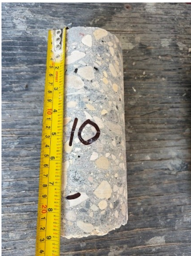
Core 10 - Mid Slab
