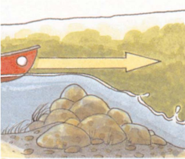
Figure 5: The stone structures of riffles act like dams, making a higher water level upstream of the structure.
