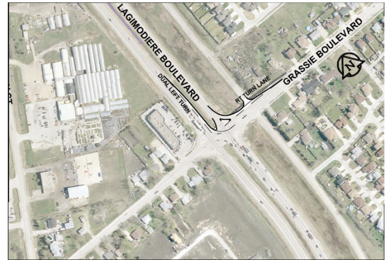
TURNING LANE ADDITIONS ON LAGIMODIERE BOULEVARD AND GRASSIE BOULEVARD
