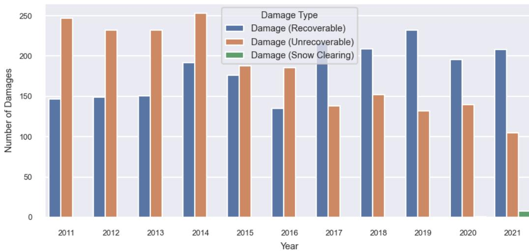
Figure 11: Number of recoverable and unrecoverable traffic signal damages, by year (2011-2021)
