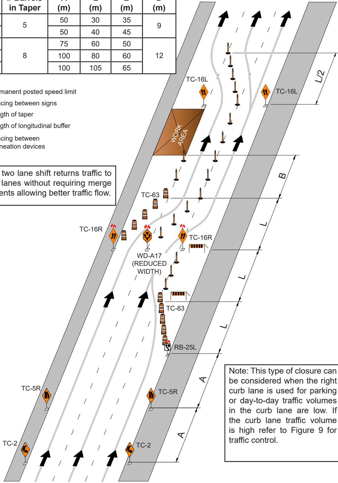
Note: This type of closure can be considered when the right curb lane is used for parking or day-to-day traffic volumes in the curb lane are low. If the curb lane traffic volume is high refer to Figure 9 for traffic control.
