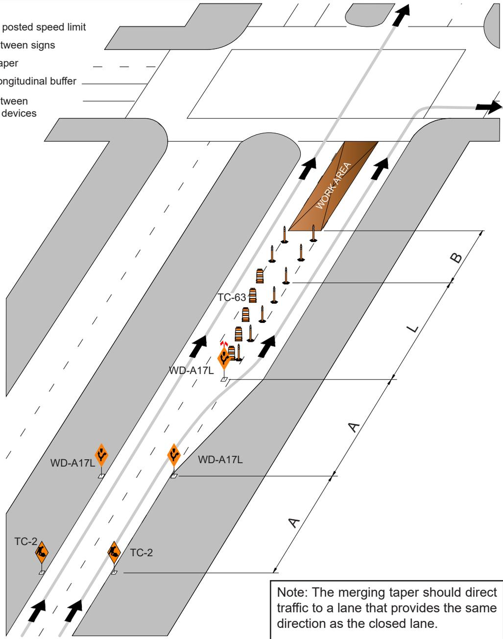
Note: The merging taper should direct traffic to a lane that provides the same direction as the closed lane.
