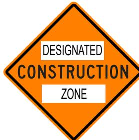
If the DCZ is located in the City's Bilingual Signing Area, as outlined in Section 3.02, the bilingual version of the 'Designated Construction Zone' (MC-1DB) sign must be used (minimum size 900 mm x 900 mm).
