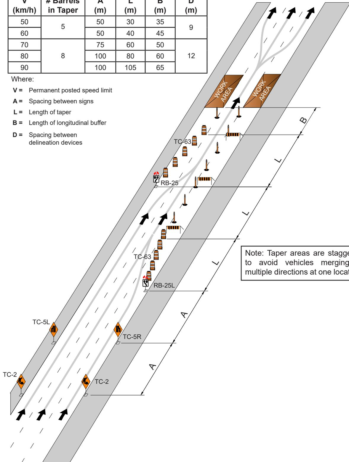
Note: Taper areas are staggered to avoid vehicles merging in multiple directions at one location.
