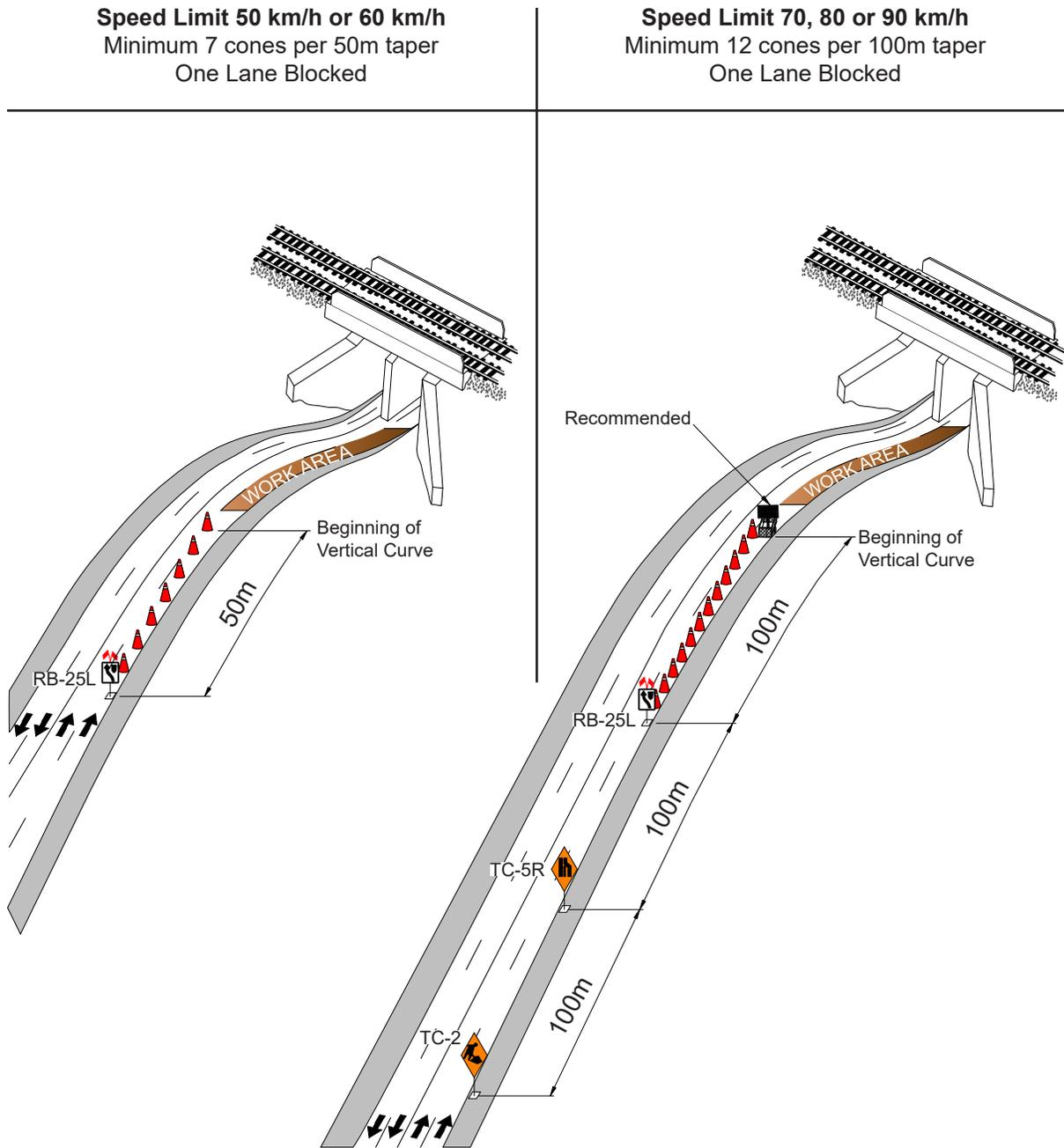
Note: Short term closures may not be used at night without written consent from the Traffic Management Branch ([PWDLaneClosures@winnipeg.ca](mailto:PWDLaneClosures@winnipeg.ca)). Use of a flashing or sequential arrow traffic control device is a requirement for work at night.
