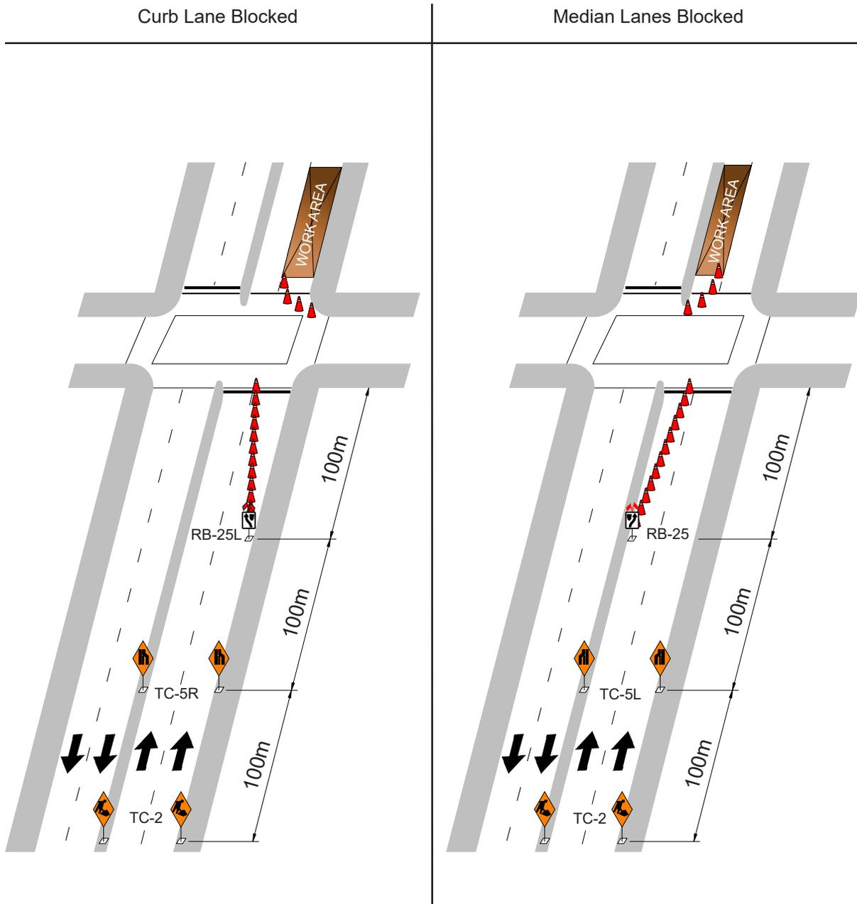
Note: Short term closures may not be used at night without written consent from the Traffic Management Branch ([PWDLaneClosures@winnipeg.ca](mailto:PWDLaneClosures@winnipeg.ca)). Use of a flashing or sequential arrow traffic control device is a requirement for work at night.
