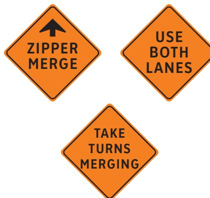
The “Take turns merging” sign can also be replaced by a single VMS.
