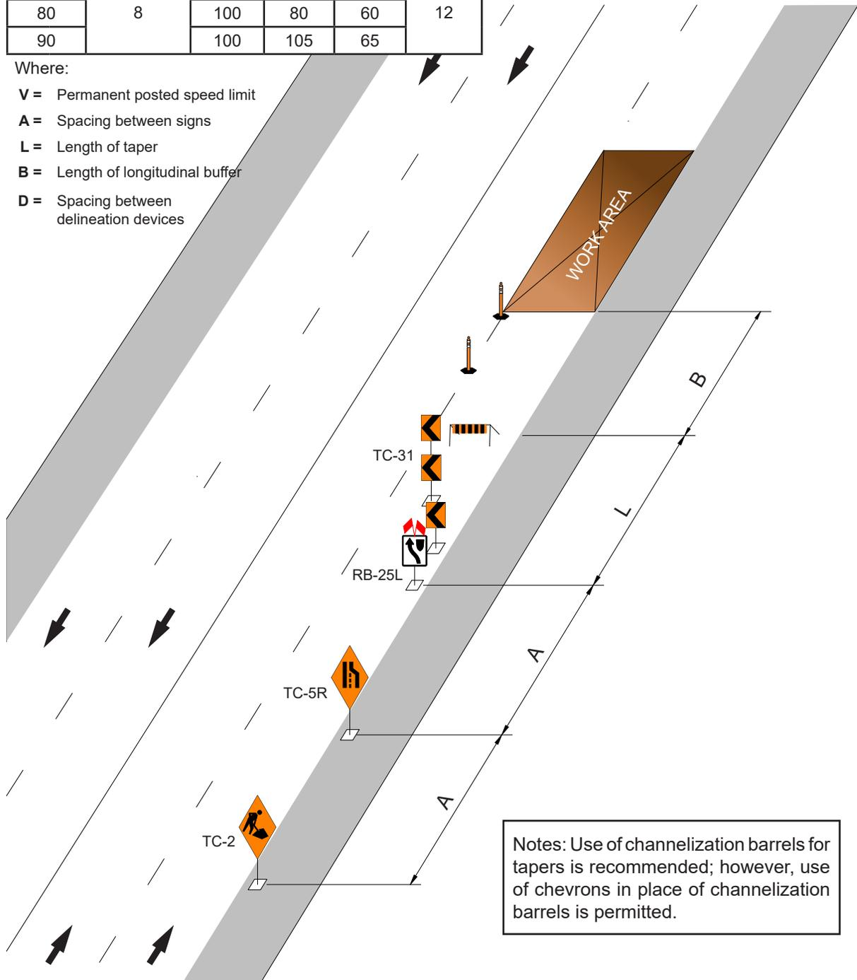
Notes: Use of channelization barrels for tapers is recommended; however, use of chevrons in place of channelization barrels is permitted.
