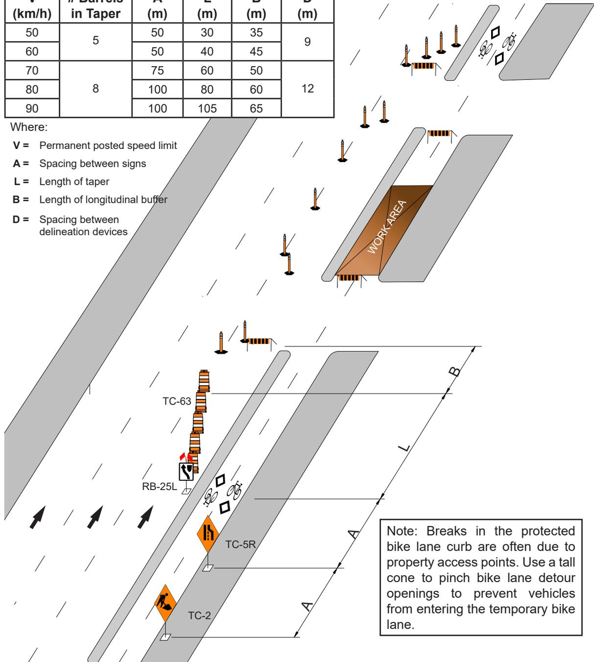
Note: Breaks in the protected bike lane curb are often due to property access points. Use a tall cone to pinch bike lane detour openings to prevent vehicles from entering the temporary bike lane.
