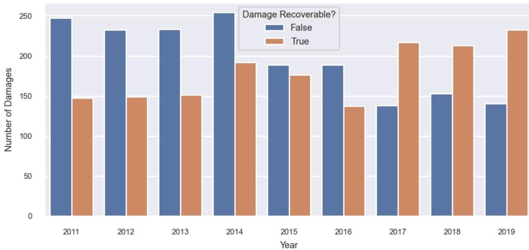
Figure 12: Number of recoverable and unrecoverable traffic signal damages, by year (2011-2019)
