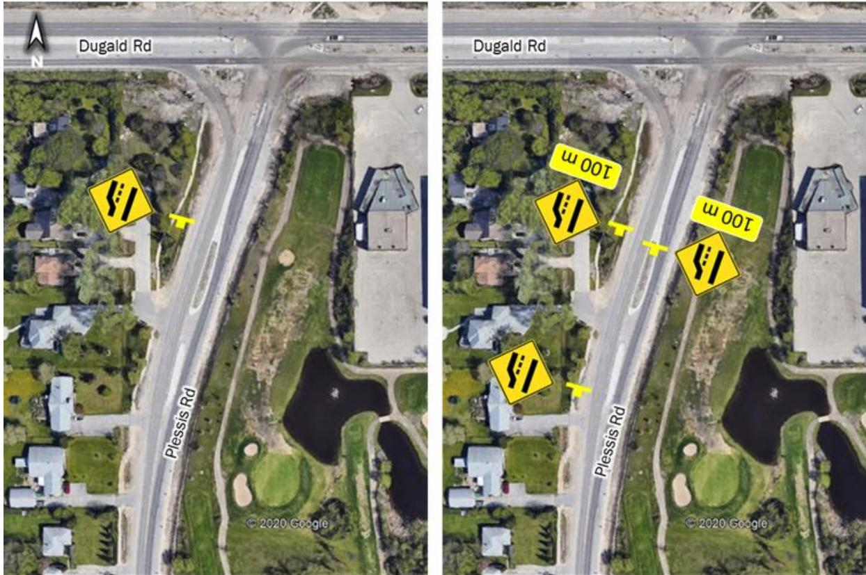
**Figure 1: Existing and Proposed “right lane ends” signage**
