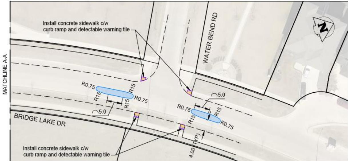
**Figure 6: Median Design at Water Bend Road (North Leg)**
