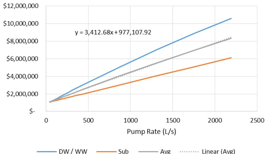
Figure 9-3. High Flow Lift Station Construction Cost Curve
