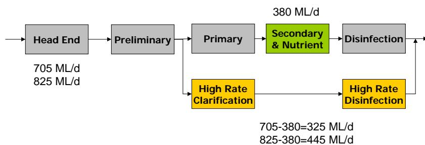
Figure 7-18. NEWPCC Process Flow Schematic
