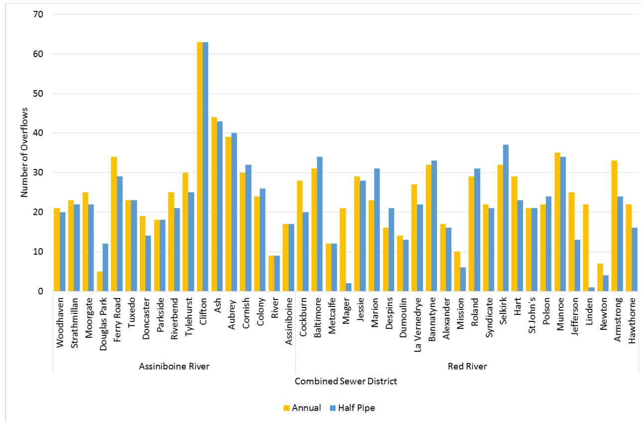
Figure 7-12. CSO Frequency with Control Gate at Half Pipe – 1992 Representative Year
