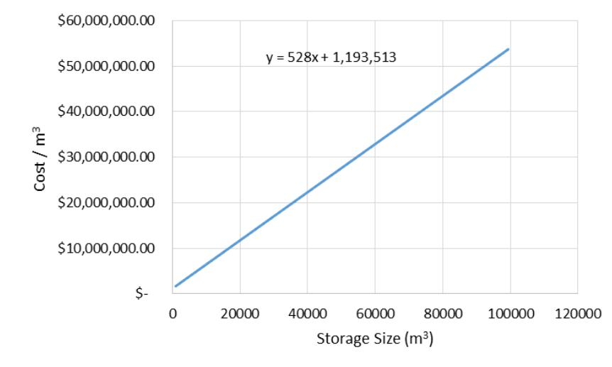
Figure 9-4. Off-line Storage Construction Cost Curve
