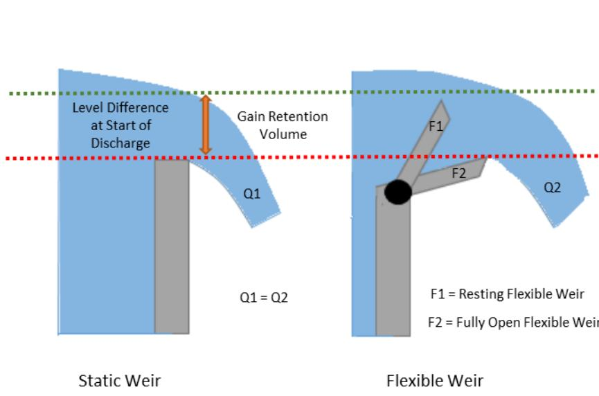
Figure 7-8. Flexible Weir vs Static Weir Schematic
