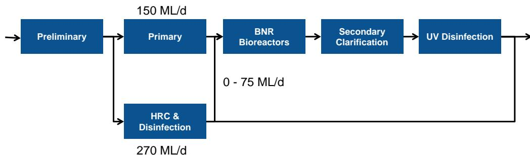
Figure 7-20. SEWPCC Process Flow Schematic
