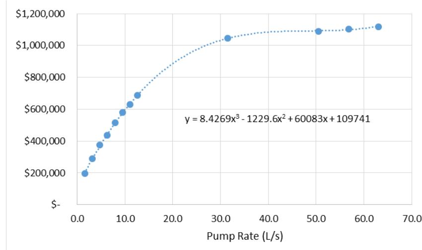
Figure 9-2. Low Flow Lift Station Construction Cost Curve
