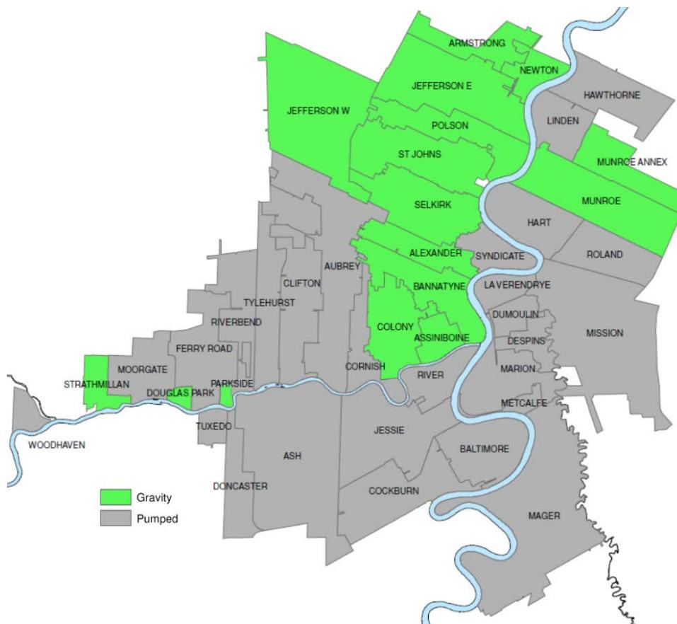
Figure 2-5. Combined District Conveyance Type – Gravity or Pumped
