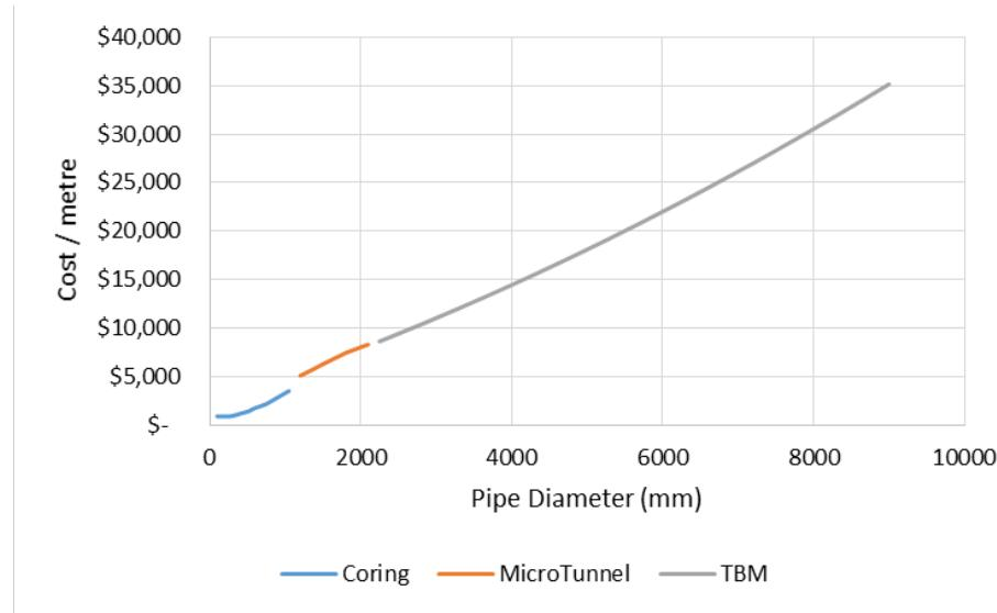
Figure 9-1. Gravity Sewer Construction Cost Curve
