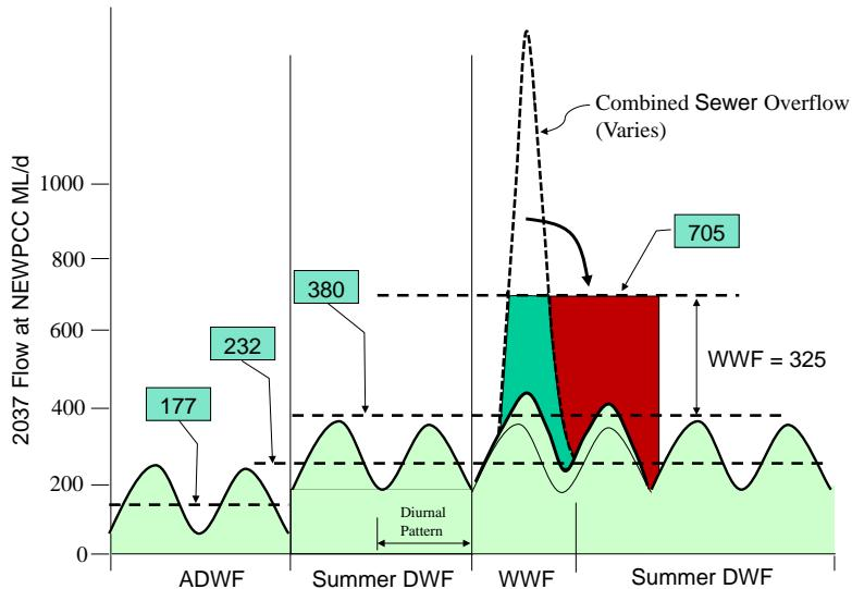
Figure 7-19. 2037 NEWPCC Flow Schematic for 705 ML/d
