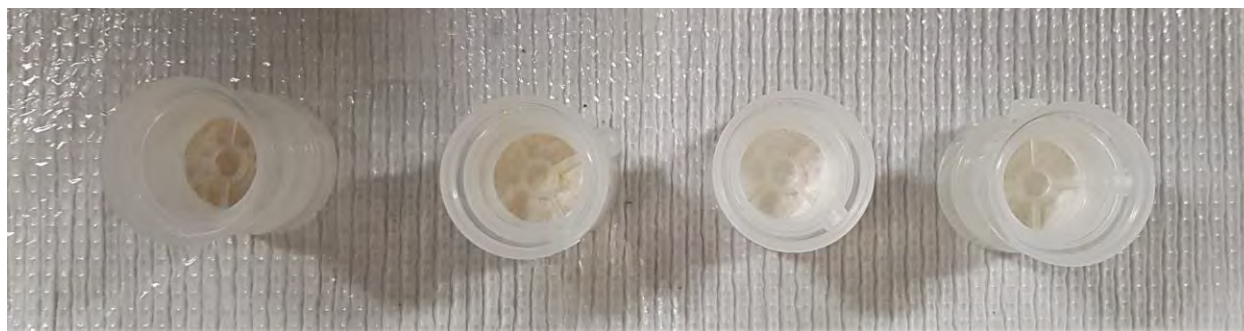
Figure 5-15: Disposable filters used to isolate dissolved fractions for analytical testing by the City Lab. Disposable filters (left to right) were used for samples collected from the individual filter effluents (Filters 1-4). A yellow precipitate was observed on the filter paper after they were used.
