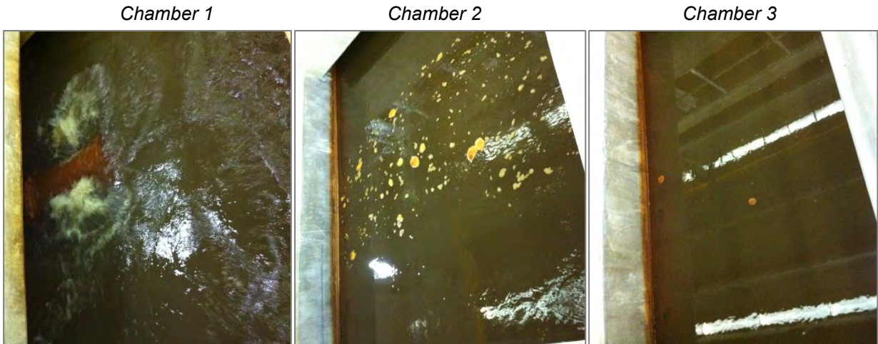
Figure 2-2: Typical particle settling by flocculation chambers, chambers 1 to 3, from left to right.
