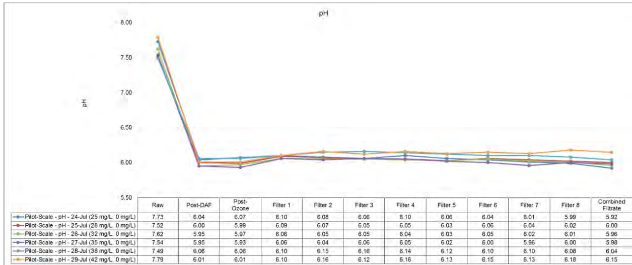
Figure 5-7: pH during the Summer piloting session for determining the optimal dose of ferric sulphate. Data originates from benchtop analysis using a Thermo Scientific Orion Star A325 pH probe.
