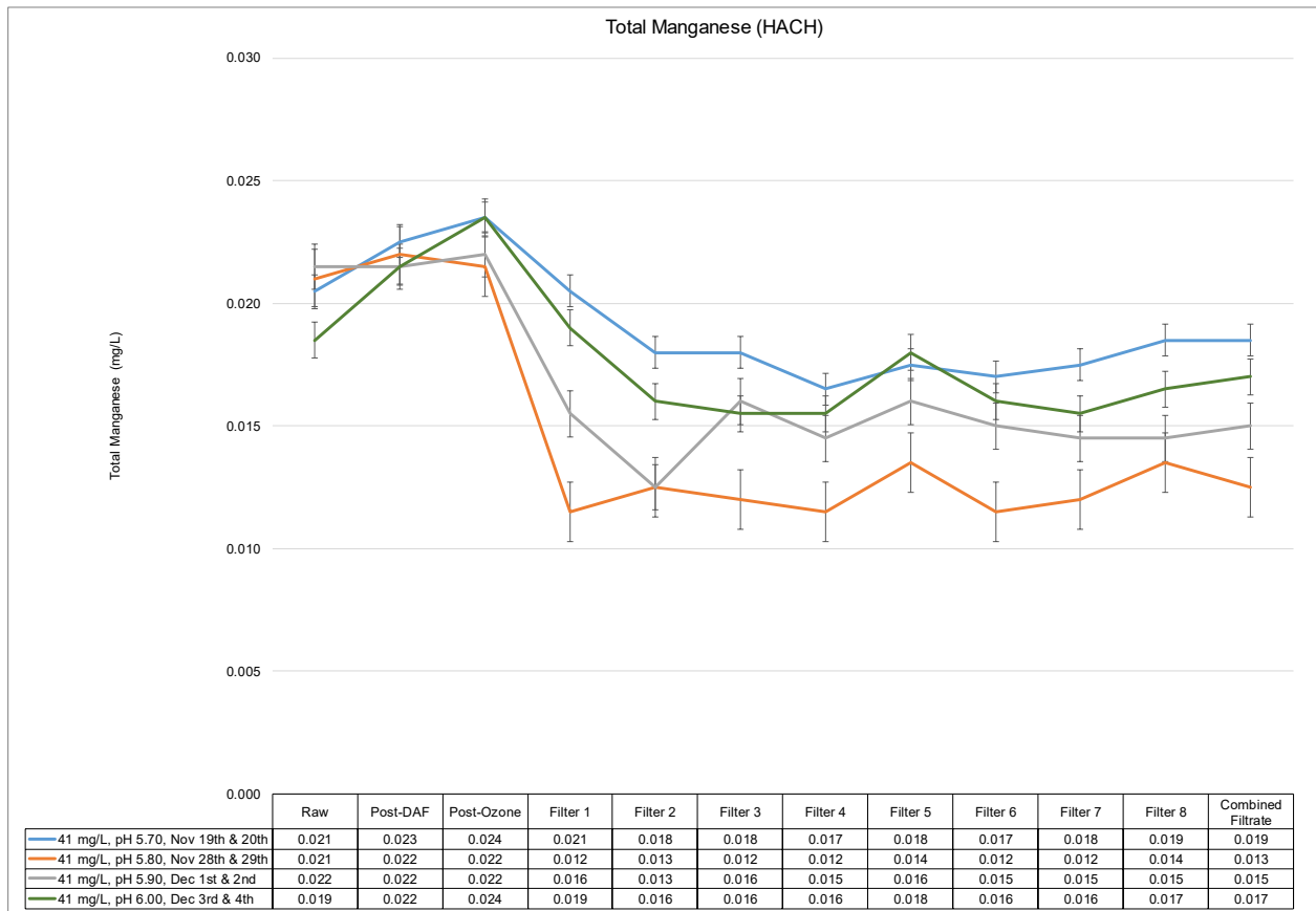
Figure 4-16: Total manganese measured following pilot-scale treatment processes during pH optimization for ferric sulphate during the Winter #2 piloting session. Data originates from the benchtop analysis using a HACH DR6000 UV-VIS spectrophotometer.
