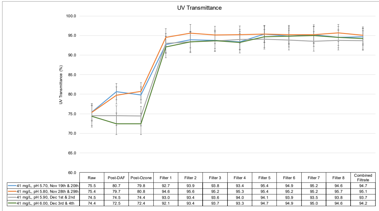
Figure 4-14: Average UVT measured following the pilot-scale system processes during pH optimization for ferric sulphate during the Winter #2 piloting session. Data originates from the benchtop analysis using a HACH DR6000 UV-VIS spectrophotometer.
